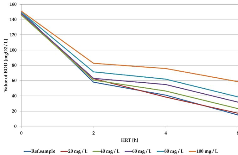
**Figure 2.** BOD removal in the bench-scale experiment (stage 1)
