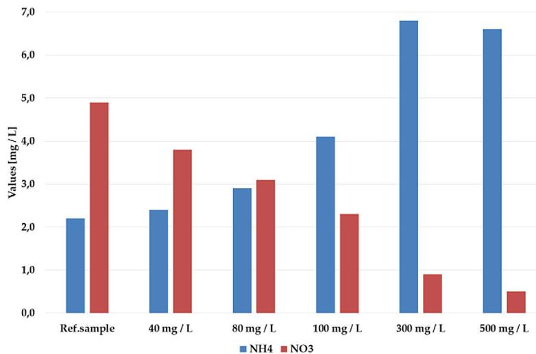
Figure 17. NH<sub>4</sub>/NO<sub>3</sub> ratio in treated water
