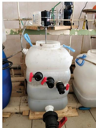
Fig. 1. Scheme and photo of the sequence batch reactor bench
