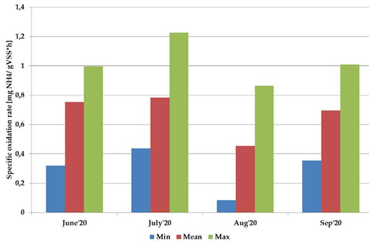
Figure 7. Specific oxidation rates (ammonia) at real WWTP
