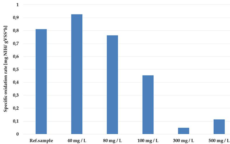
Figure 15. Mean values of specific oxidation rates (ammonia) at bench-scale
