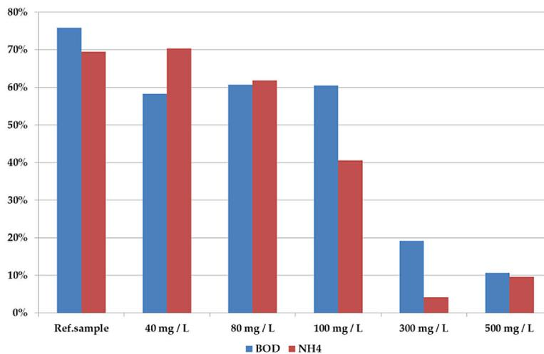
Figure 14. Mean efficiency of ammonia and BOD removal
