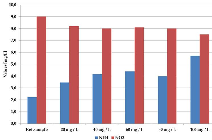
Figure 9. NH<sub>4</sub>/NO<sub>3</sub> ratio in the effluent
