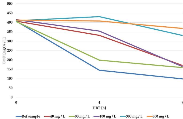
Figure 12. BOD removal in the bench-scale experiment (stage 2)
