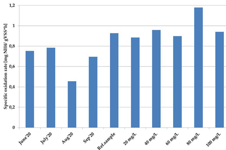
Figure 8. Mean values of specific oxidation rates (ammonia) at bench-scale and full-scale experiment
