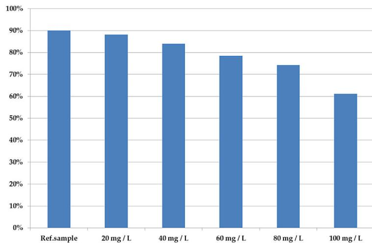
**Figure 3.** Mean values of efficiency of bench-scale BOD removal
