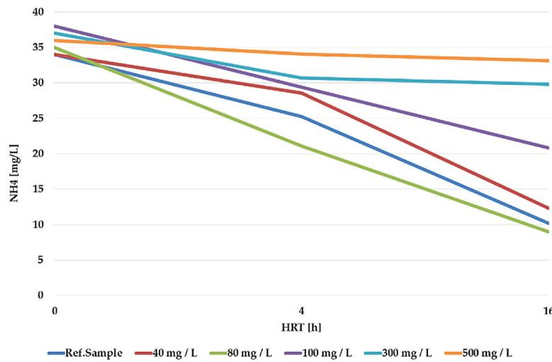
Figure 13. Ammonia removal in the bench-scale experiment (stage 2)
