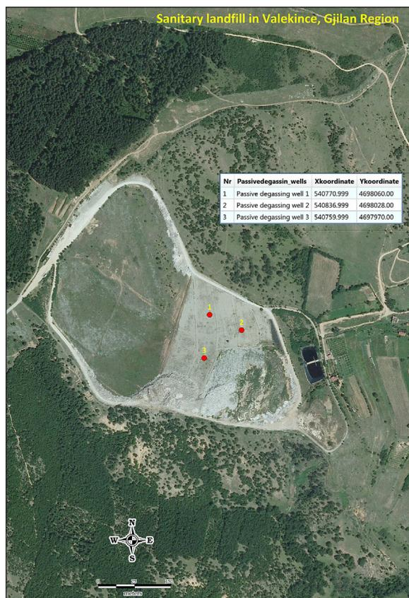
Figure 6. Monitoring sites of methane concentration in the sanitary landfill Velekince
