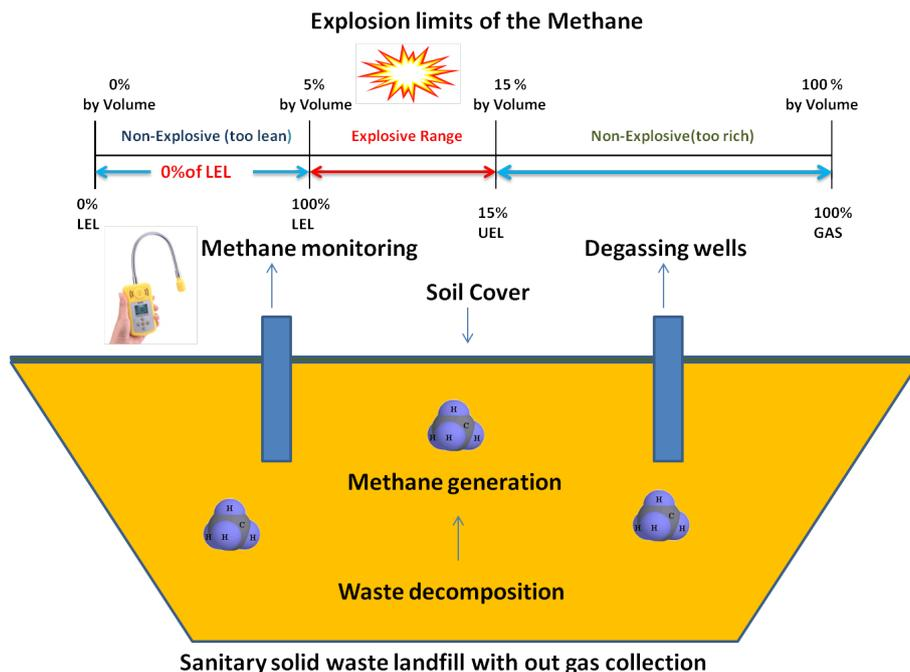
**Figure 5.** The methane concentration monitoring scheme in a landfill without gas collection
