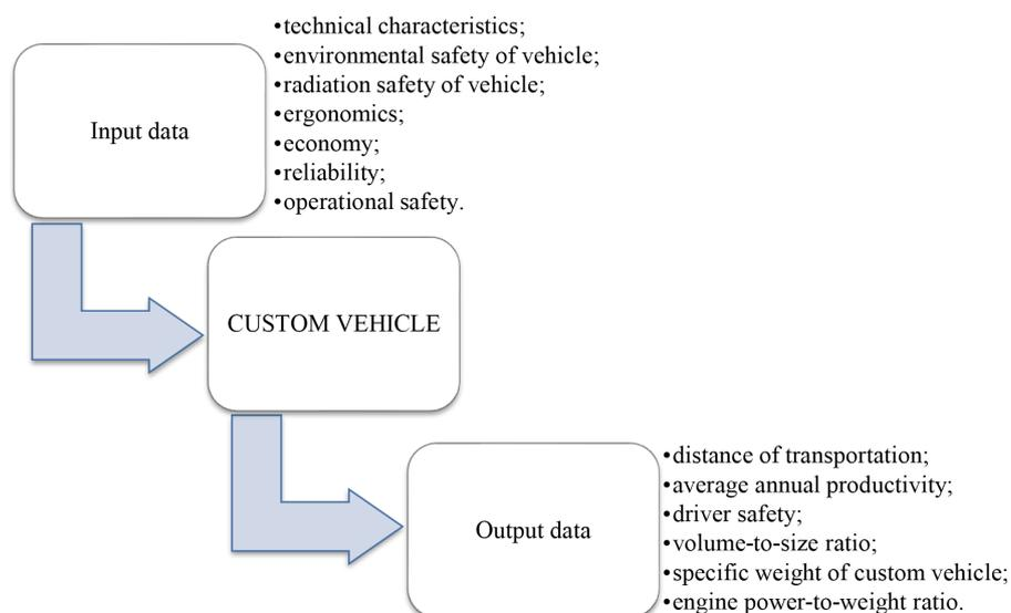
**Figure 1.** Requirements for custom vehicles that transports household and hazardous waste at the “entrance” and “exit” of the environmental logistics system
