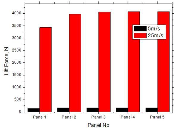
**Figure 16.** Comparison of lift forces on row1 of the hexagonal panel of farm with the variation in the wind velocity on the back face
