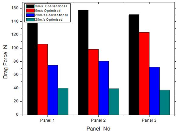
**Figure 7.** Effect of drag force on different panels and models of the panels at 135° angle of orientation
