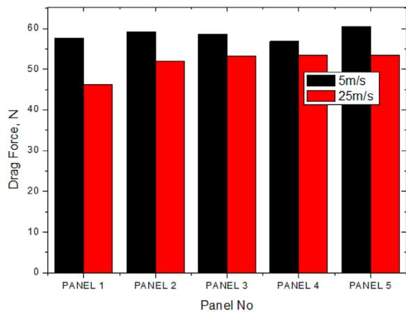
**Figure 12.** Comparison of drag forces on row 1 of the hexagonal panel of solar farm with the variation in the wind velocity on rear face
