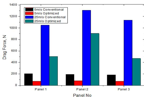
Figure 5. Effect of drag force on different panels and models of the panels at 0° angle of orientation
