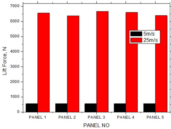
**Figure 13.** Comparison of lift forces on row1 of the rectangular panel of farm with the variation in the wind velocity on the front face
