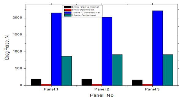
Figure 6. Effect of drag force on different panels and models of the panels at 45° angle of orientation
