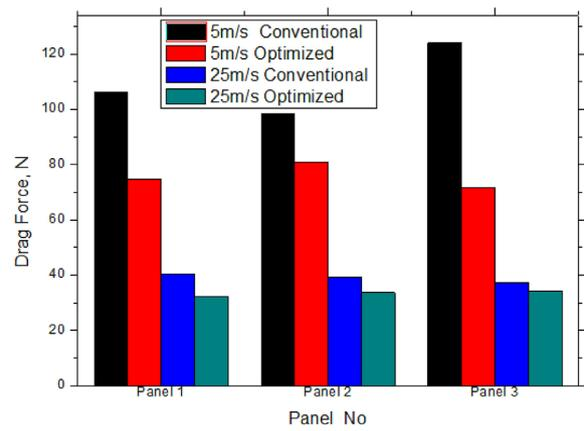
**Figure 8.** Effect of drag force on different panels and models of the panels at 180° angle of orientation
