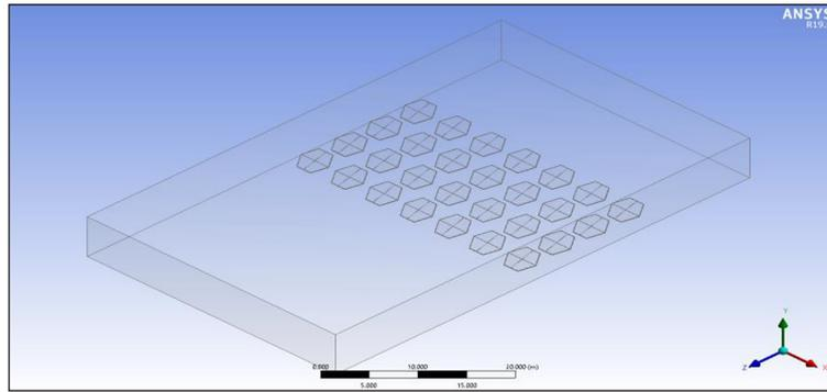
**Figure 2.** Numerical model of Optimized hexagonal shaped panels mounted on the ground
