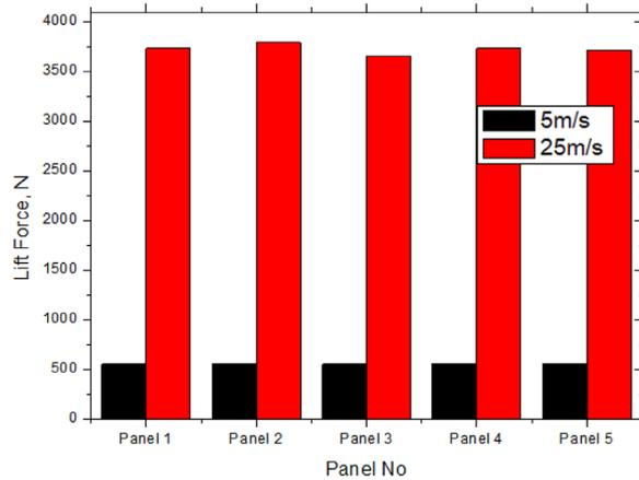
**Figure 14.** Comparison of lift forces on row1 of the rectangular panel of farm with the variation in the wind velocity on the back face
