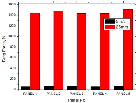
**Figure 11.** Comparison of drag forces on row1 of the hexagonal panel of farm with the variation in the wind velocity on the front face
