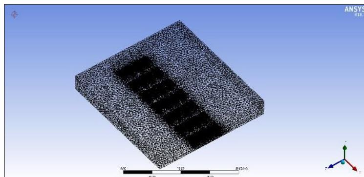
**Figure 3.** Meshed model of the traditional ground mounted solar panel array
