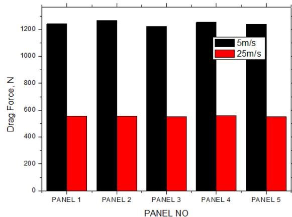
**Figure 10.** Comparison of drag forces on row1 of the rectangular panel of farm with the variation in the wind velocity on the back face
