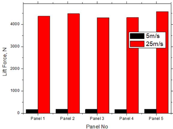
**Figure 15.** Comparison of lift forces on row1 of the hexagonal panel of farm with the variation in the wind velocity on the front face
