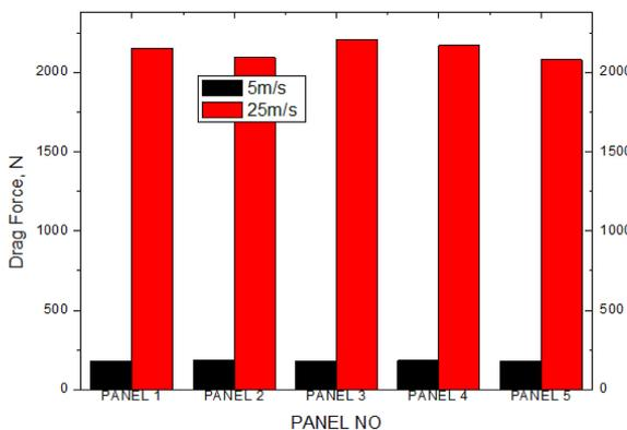
**Figure 9.** Comparison of drag forces on row1 of the rectangular panel of farm with the variation in the wind velocity on the front face
