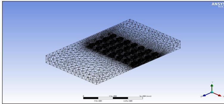
Figure 4. Meshed model of optimized hexagonal solar panel array
