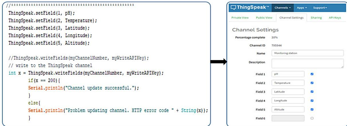
Figure 9. Configuration of the fields in the communication channel with the web server
