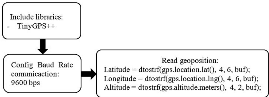
Figure 7. Latitude, longitude and altitude measurement flow chart with GPS NEO 6M
