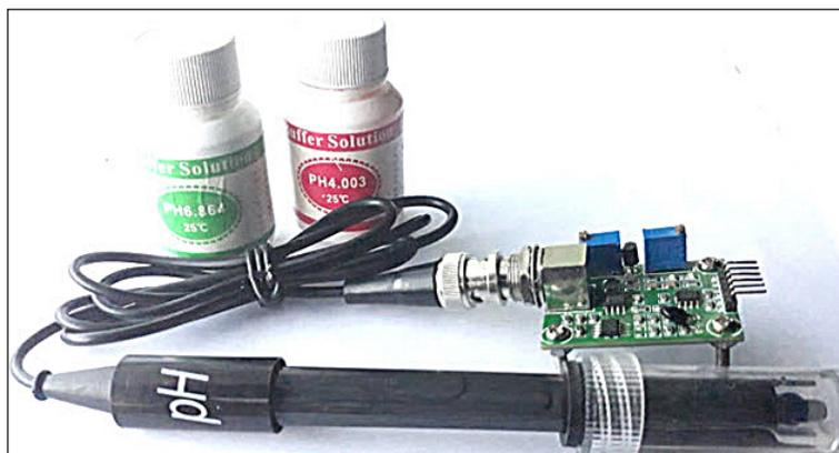
**Figure 3.** PH meter calibration module, probe and buffers
