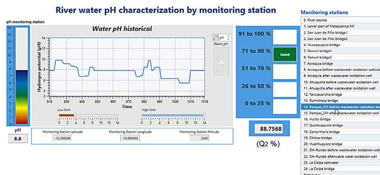
**Figure 15.** Interface for monitoring and characterizing the pH of river waters with data from the cloud
