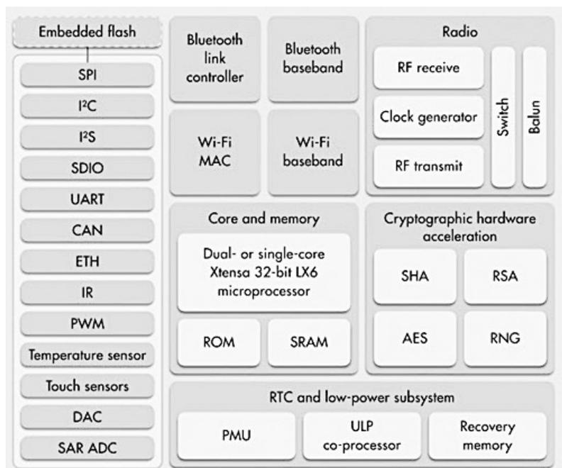
Figure 8. ESP32 processor function diagram
