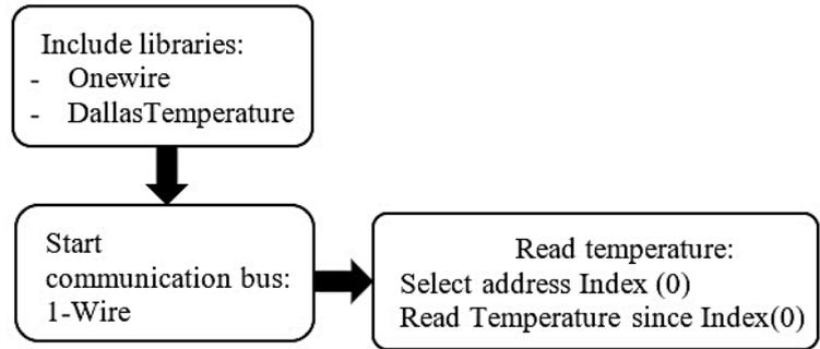
Figure 6. Temperature measurement flow chart with DS18B20 sensor
