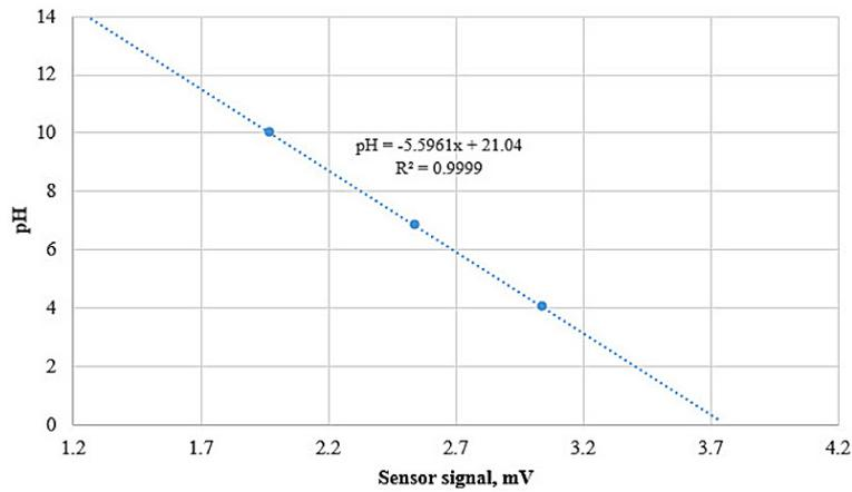
Figure 4. Three-point pH sensor calibration curve
