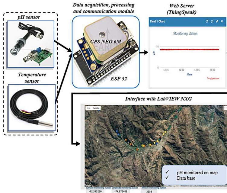
**Figure 2.** General diagram of the electronic data collection and analysis system
