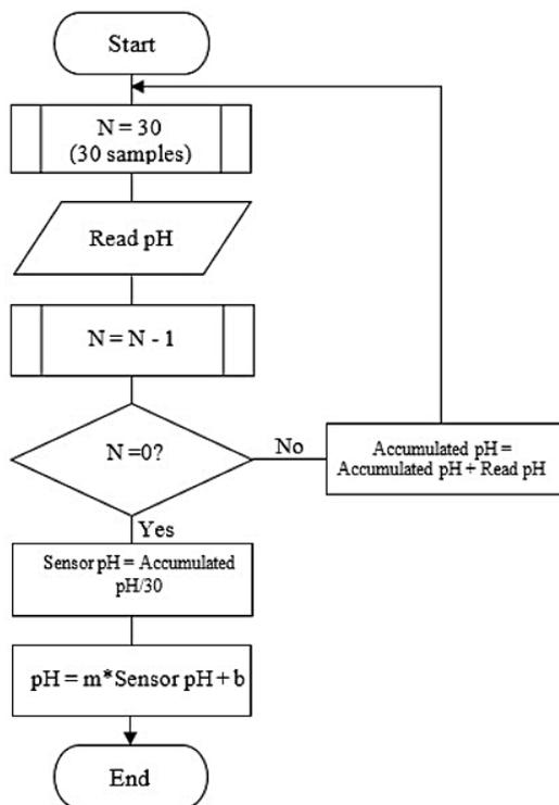
Figure 5. PH sensor measurement flow chart
