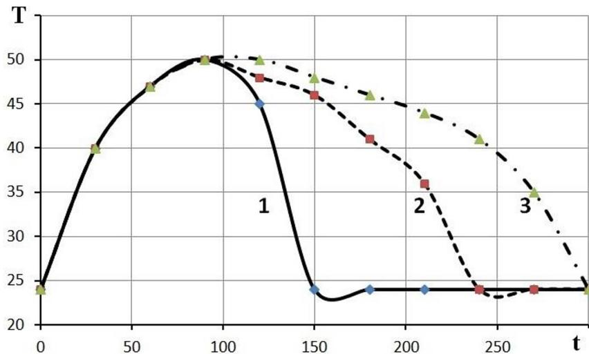
**Figure 6.** Dynamics of temperature ( $T$ , °C) at the outlet of the experimental solar collector during the simulation of clouds ( $t$ , min.) 1 – without accumulator; 2, 3 – with accumulator, without thermal insulation and heat-insulated, respectively
