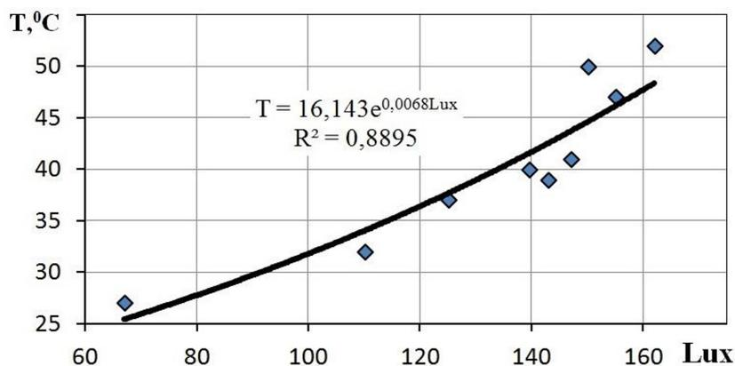
**Figure 5.** Dependence of the heating of the coolant (T, °C) on the illumination of the collector surface (Lux\*1,000)
