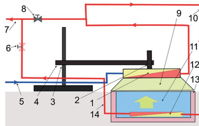
**Figure 3.** View of solar installation in the presence of clouds (Kostenko et al., 2020): 1 – sealed housing, 2 – bracket, 3 – riser, 4 – rail, 5 – pipe, 6 – valve, 7 – pipe, 8 – valve, 9 – casing, 10 – pipe, 11 – heat accumulator, 12 – heat exchanger, 13 – thermal insulation layer, 14 – pipe
