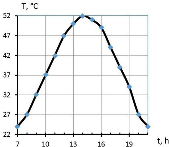
**Figure 4.** Dynamics of temperature (T, °C) at the outlet of the experimental solar collector during daylight hours (t, h), 25.07.2020
