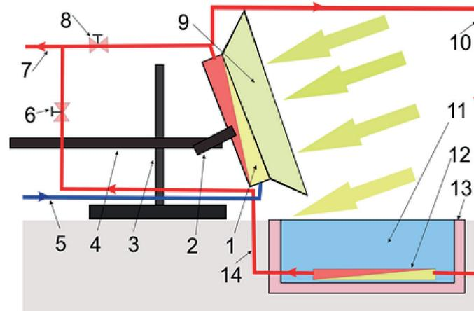
**Figure 2.** View of solar installation in the “recharge” mode of the accumulator (Kostenko et al., 2020): 1 – sealed housing, 2 – bracket, 3 – riser, 4 – rail, 5 – pipe, 6 – valve, 7 – pipe, 8 – valve, 9 – casing, 10 – pipe, 11 – heat accumulator, 12 – heat exchanger, 13 – thermal insulation layer, 14 – pipe
