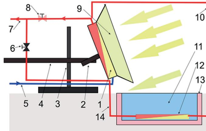
**Figure 1.** View of solar installation in normal sunlight (Kostenko et al., 2020): 1 – sealed housing, 2 – bracket, 3 – riser, 4 – rail, 5 – pipe, 6 – valve, 7 – pipe, 8 – valve, 9 – casing, 10 – pipe, 11 – heat accumulator, 12 – heat exchanger, 13 – thermal insulation layer, 14 – pipe
