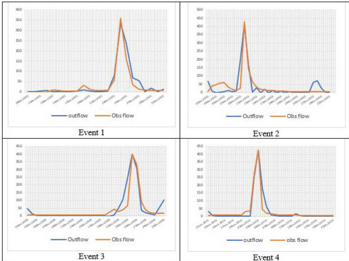
Figure 6. Simulated and observed hydrographs during calibration
