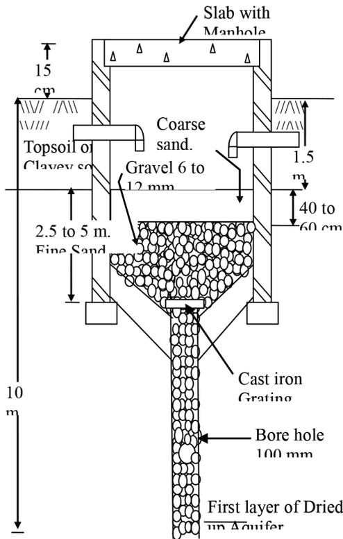
Figure 3. Recharge Bore-Well
