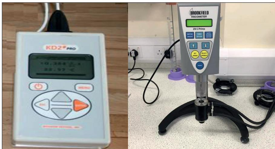
**Figure 5.** Photographs of (a) Kd2 pro thermal analyzer, (b) Brookfield viscometer
