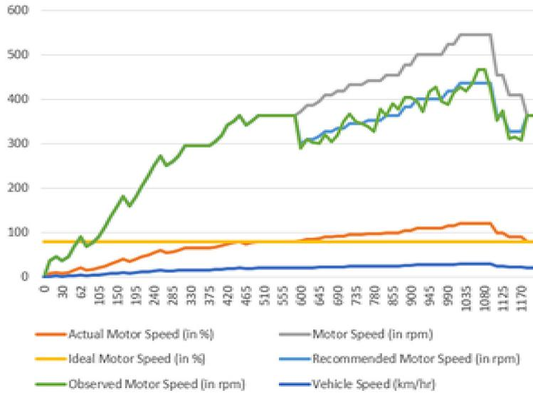
Fig. 8. Speed Control based on motor speed (in rpm)
