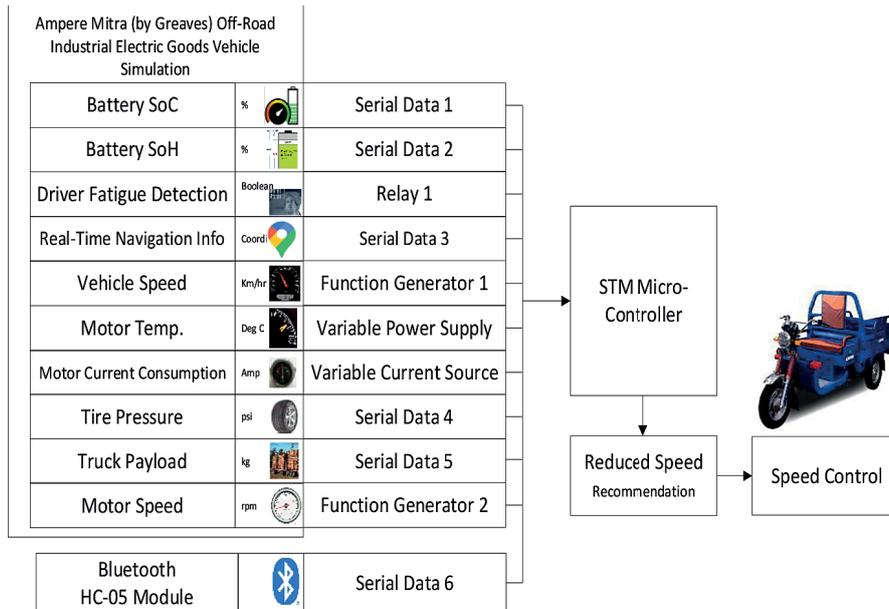
Fig. 6. Simulation and testing block diagram
