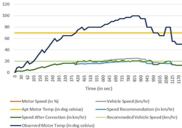
Fig. 9. Speed control based on motor temp
