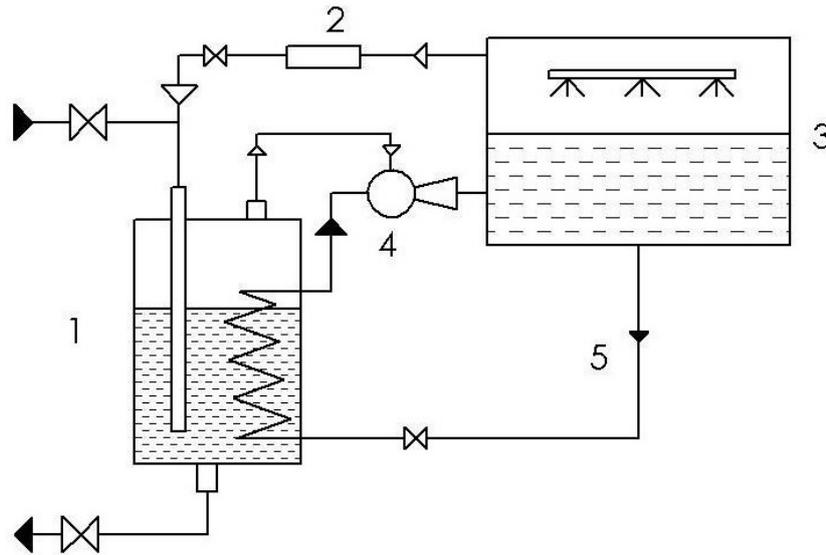
**Figure 1.** Diagram of the installation of periodic physical absorption for an aqueous copper-puddle outlet. 1 – physical desorber, 2 – filter, 3 – pickling machine, 4 – quarterly, 5 – pump.
