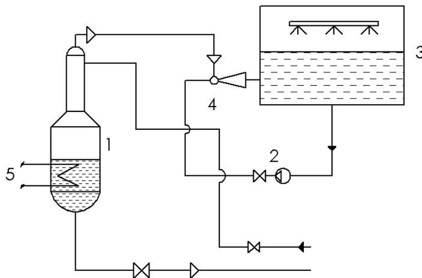
**Figure 2.** Diagram of the simple distillation installation: 1 – Alembic; 2 – pump; 3 – etching machine; 4 – jet pump (injector); 5 – electric heater.
