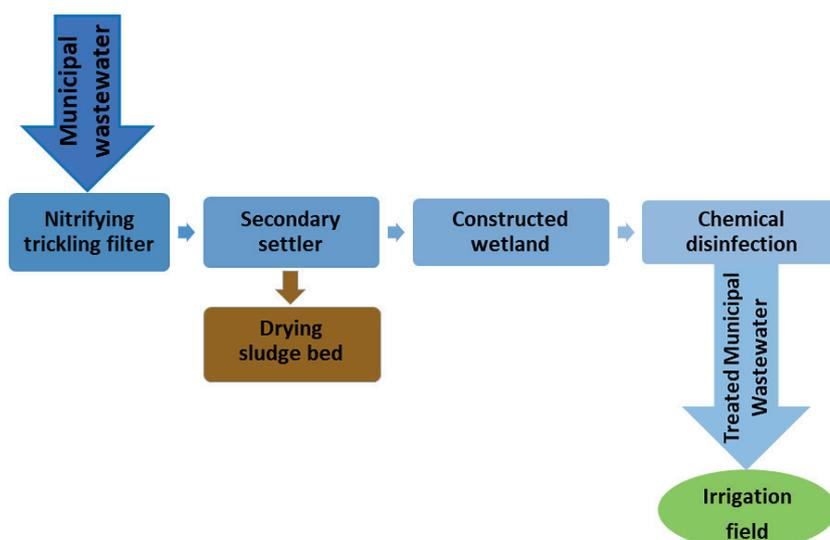
**Figure 3.** The municipal wastewater treatment process
