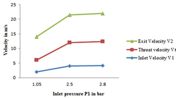
Fig.7. Pressure distribution vs velocities
