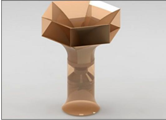
Fig. 3. Pro-E Model of venturi wind mill
