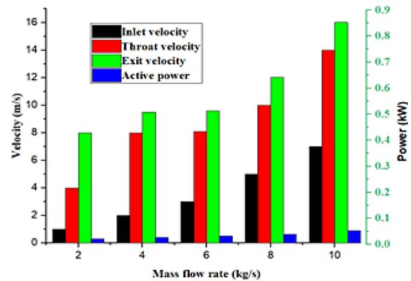
Fig. 10. Distribution of wind velocity over the venturi wind turbine
