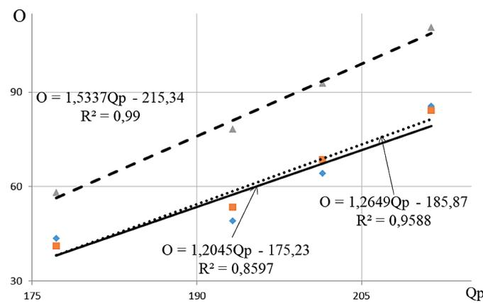
**Figure 5.** Effective set-up rate ( $O$ ) when changing the operating modes of the compressor ( $Q_p$ ,  $m^3/s \cdot 10^{-6}$ ). Solid, dotted, dashed lines – design options I, II, III, respectively
