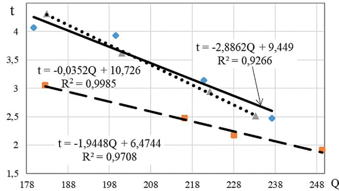
**Figure 4.** Time ( $t$ , s) of travel of bubbles through two stages at different operating modes of the set-up ( $Q_p$ ,  $m^3/s \cdot 10^{-6}$ ). Solid, dotted, dashed lines – design options I, II, III, respectively
