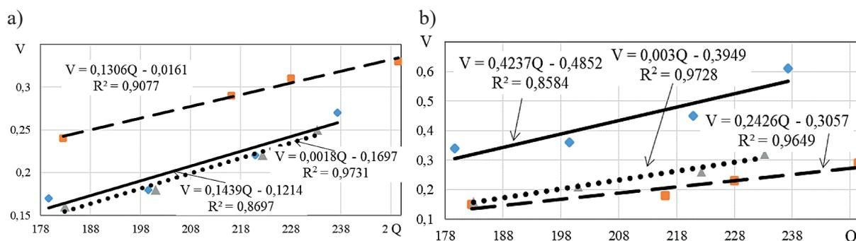
**Figure 3.** Velocity of air bubbles ( $V$ , m/s) in the mixing chamber (a) and the airlift column (b) depending on the performance of the set-up ( $Q_p$ ,  $m^3/s \cdot 10^{-6}$ ). Solid, dotted, dashed lines – respectively I, II, III options of the airlift design
