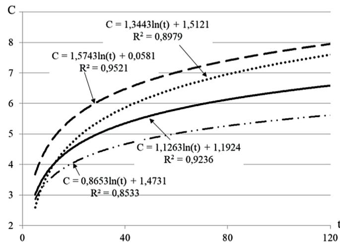
**Figure 6.** Dynamics of water oxygenation ( $C$ , mg/L). Solid, dotted, dashed lines – liquid supply by airlift ( $Q_p$ ,  $m^3/s \cdot 10^{-6}$ ), respectively, 6.25, 7.72 and 22.86, dashed-dotted line – conventional aerator, ( $t$ , min) duration of aeration,
