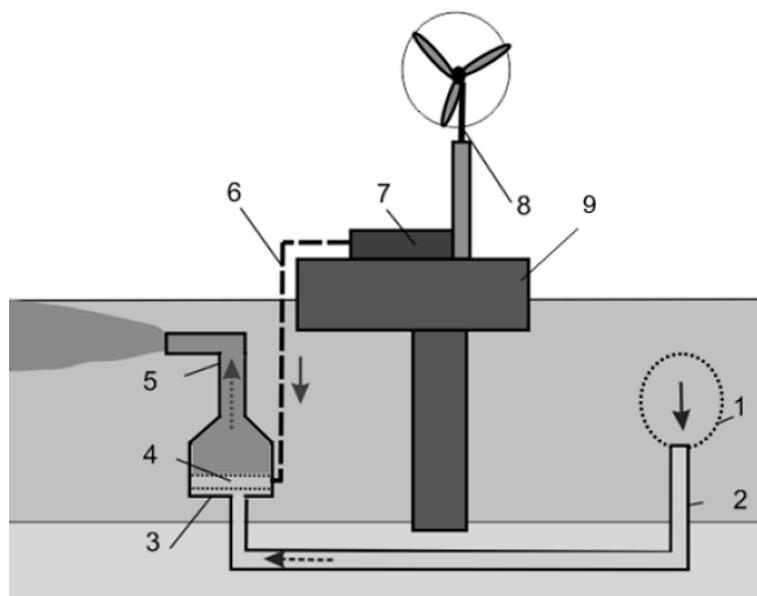
**Figure 1.** Schematic construction of the airlift aerator: 1 – strainer; 2 – geothermal heat exchanger; 3 – mixing chamber; 4 – spray nozzle; 5 – airlift; 6 – air duct; 7 – compressor; 8 – wind turbine; 9 – foundation
