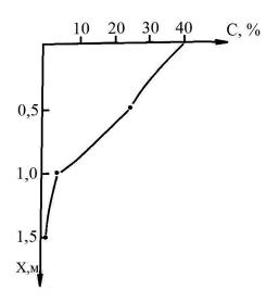
Figure 1. Salt profile after 10 years of storage etching salts of printed circuit boards
