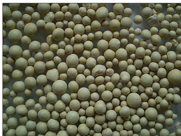
Figure 2. Appearance of the encapsulated granular ANP fertilizer with a polystyrene-lignin shell
