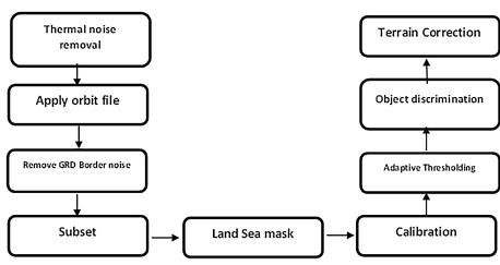
Figure 4. Chain processes of sentinel-1 image by using SNAP software
