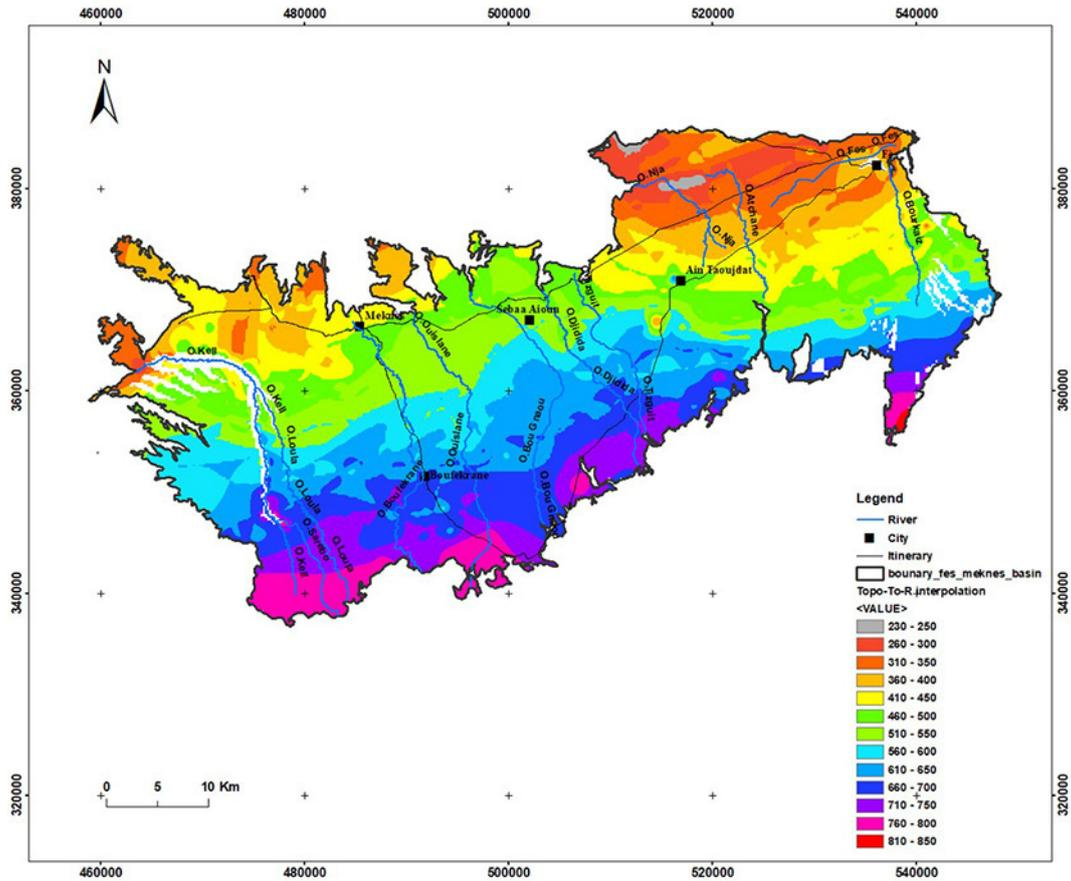
Figure 10. Map of marl bottom elevation by Topo to Raster interpolation
