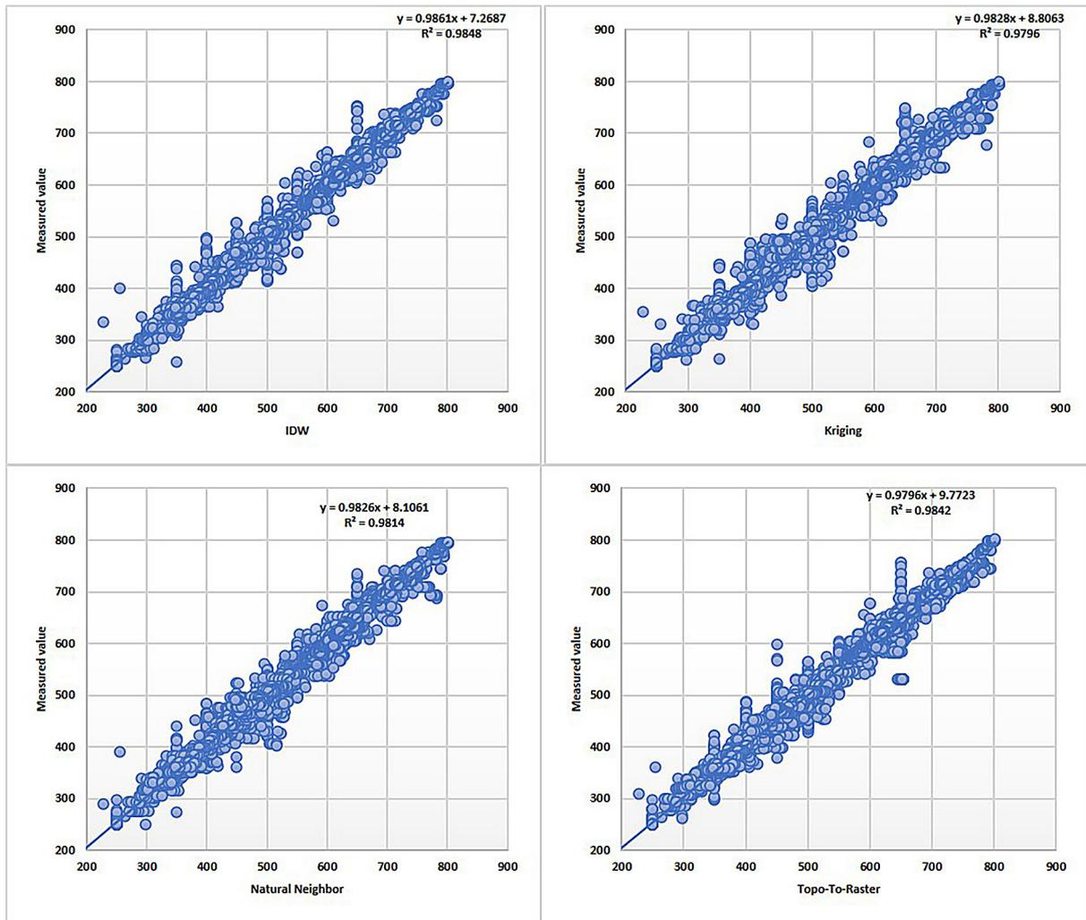
Figure 11. Linear correlation between measured and estimated marl elevations
