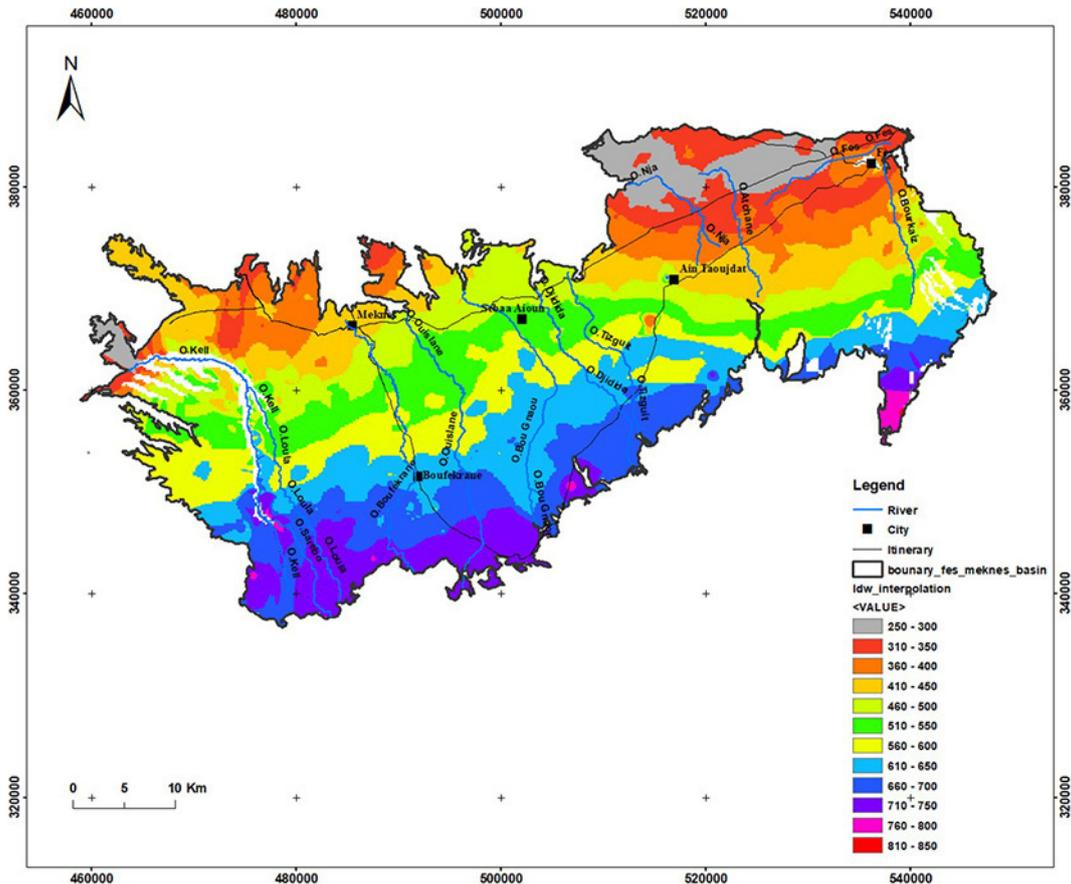
Figure 7. Map of marl bottom elevation by IDW interpolation
