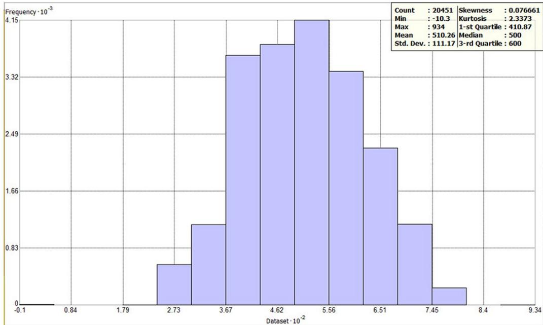
Figure 6. Frequency histogram of top elevation of the Miocene marl
