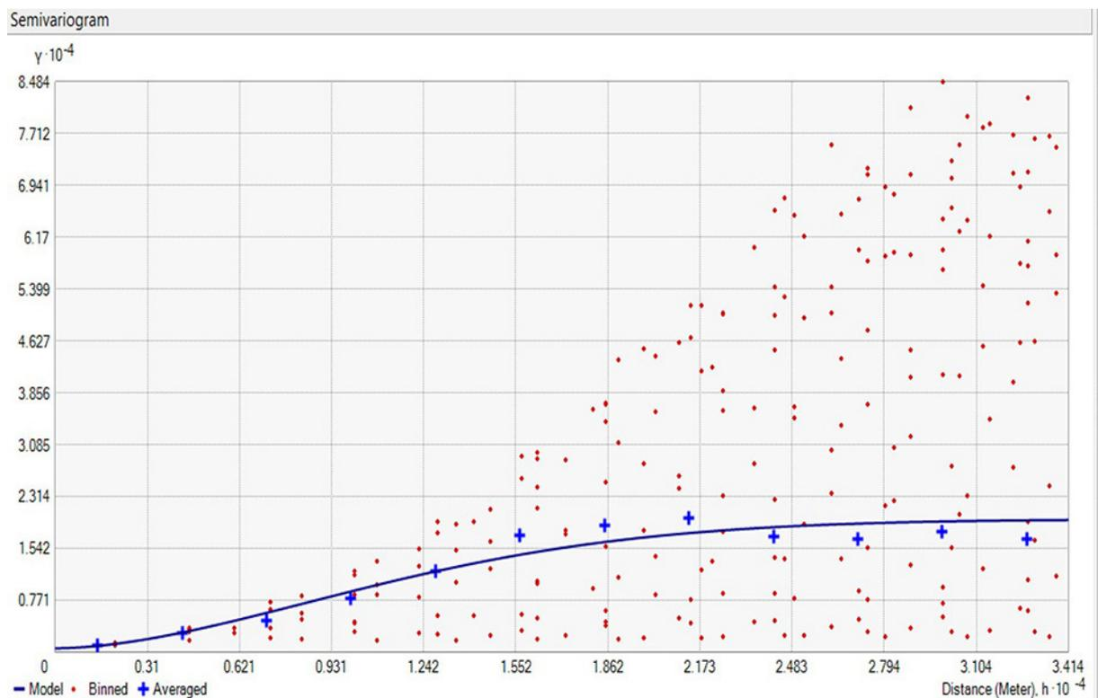
Figure 5. Semi-variogram model of the Miocene marl top elevation
