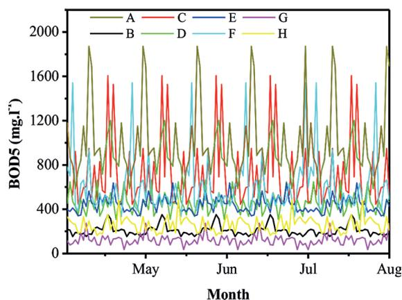
Figure 3.  $\text{BOD}_5$  concentration of raw water, lateral condition (May 01, 2019 to August 31, 2019)
