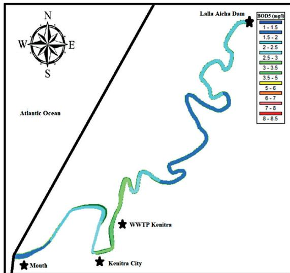
**Figure 20.** Longitudinal evolution of the BOD<sub>5</sub> in the case after installation of kenitra's WWTP at high tide (August 18, 2021)
