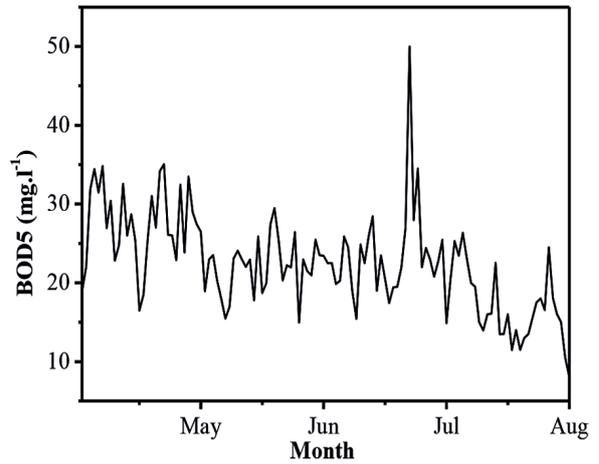
**Figure 13.** BOD5 concentration of water treated, lateral condition (May 01, 2020 to August 31, 2020)
