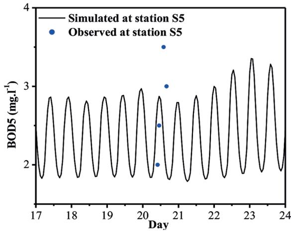
**Figure 18.** Temporal evolution of the simulated and measured of the BOD<sub>5</sub> at point 5 in the case after installation of Kenitra WWTP
