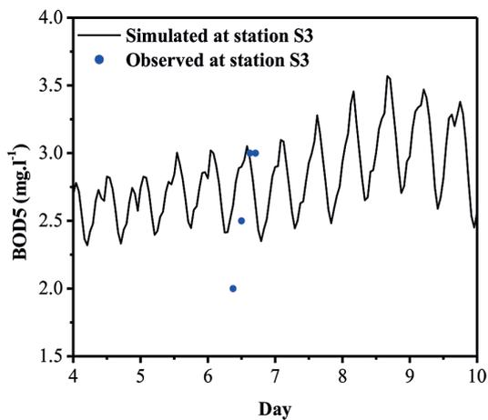
**Figure 16.** Temporal evolution of the simulated and measured of the BOD<sub>5</sub> at point 3 in the case after installation of Kenitra WWTP
