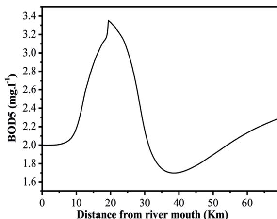
**Figure 22.** Longitudinal evolution of the BOD<sub>5</sub> in the case after installation of Kenitra's WWTP at high tide (August 22, 2021)
