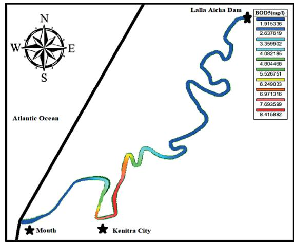
Figure 10. Longitudinal evolution of the BOD<sub>5</sub> in the case before installation of Kenitra’s WWTP at high tide (August 23, 2019)
