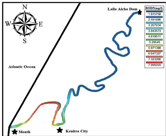
Figure 11. Longitudinal evolution of the BOD<sub>5</sub> in the case before installation of Kenitra’s WWTP at low tide (August 20, 2019)
