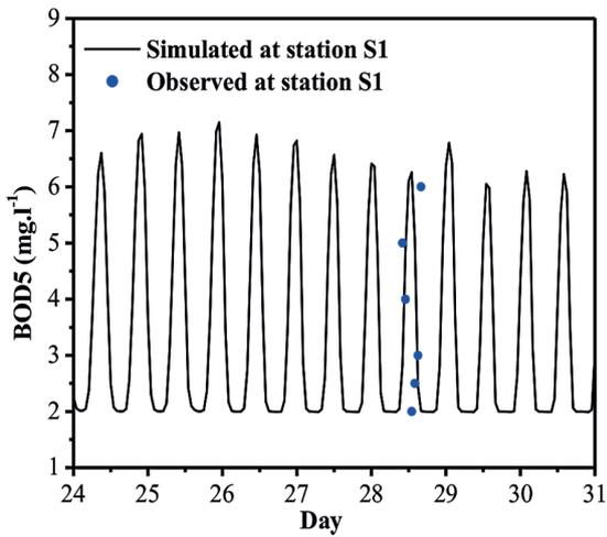
**Figure 4.** Temporal evolution of the simulated and measured of the BOD<sub>5</sub> at point 1 in the case before installation of Kenitra WWTP
