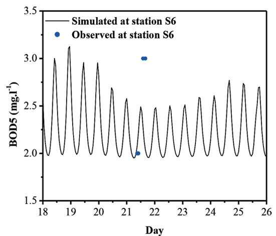
**Figure 9.** Temporal evolution of the simulated and measured of the BOD<sub>5</sub> at point 6 in the case before installation of kenitra WWTP
