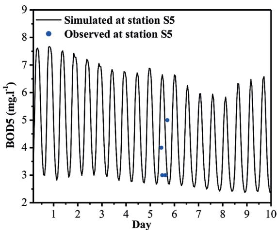
**Figure 8.** Temporal evolution of the simulated and measured of the BOD<sub>5</sub> at point 5 in the case before installation of kenitra WWTP
