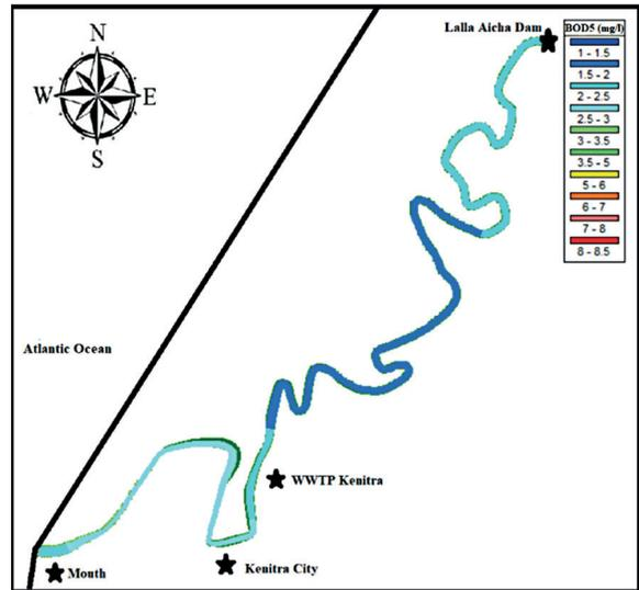
**Figure 21.** Longitudinal evolution of the BOD<sub>5</sub> in the case after installation of kenitra's WWTP at low tide (August 20, 2021)
