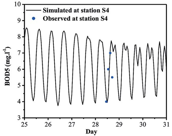
**Figure 7.** Temporal evolution of the simulated and measured of the BOD<sub>5</sub> at point 4 in the case before installation of kenitra WWTP
