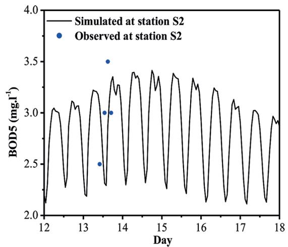
**Figure 15.** Temporal evolution of the simulated and measured of the BOD<sub>5</sub> at point 2 in the case after installation of Kenitra WWTP
