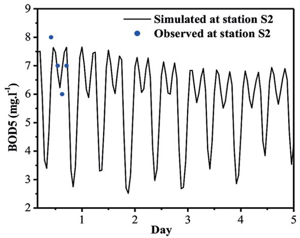
**Figure 5.** Temporal evolution of the simulated and measured of the BOD<sub>5</sub> at point 2 in the case before installation of kenitra WWTP
