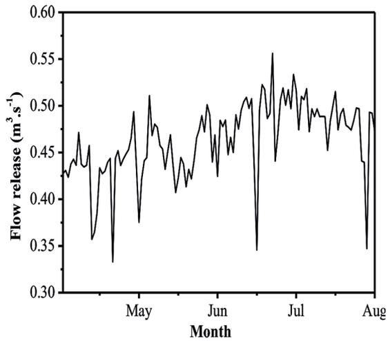
**Figure 12.** Treated water flow released by Kenitra’s WWTP (May 01, 2020 to August 31, 2020)
