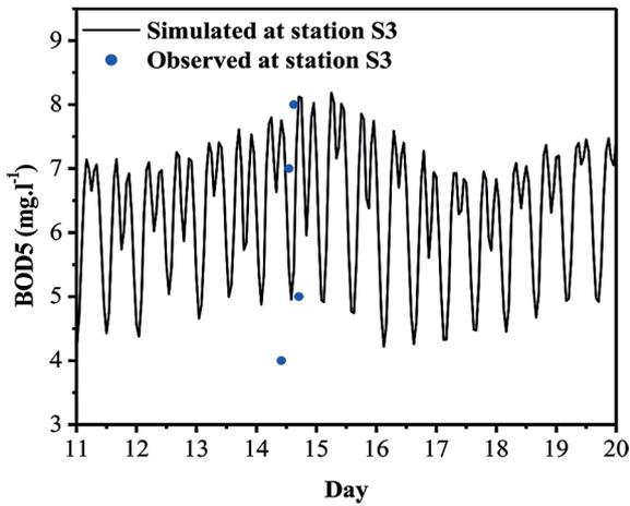
**Figure 6.** Temporal evolution of the simulated and measured of the BOD<sub>5</sub> at point 3 in the case before installation of kenitra WWTP
