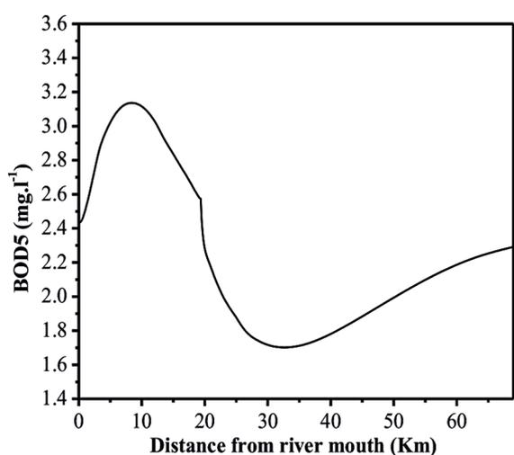
**Figure 23.** Longitudinal evolution of the BOD<sub>5</sub> in the case after installation of Kenitra's WWTP at low tide (August 22, 2021)
