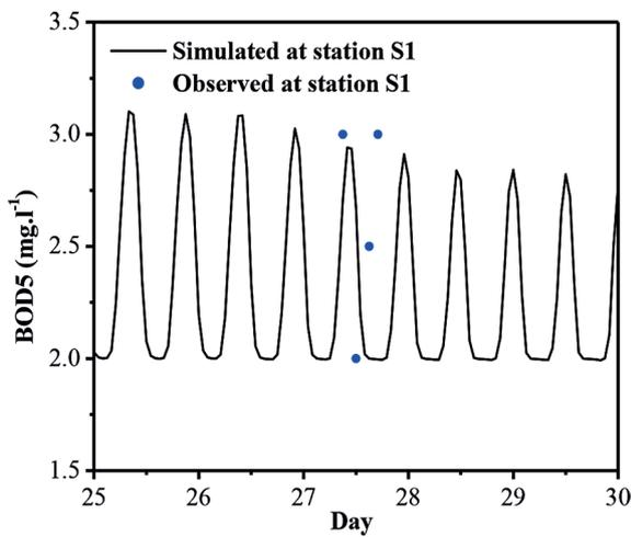
**Figure 14.** Temporal evolution of the simulated and measured of the BOD<sub>5</sub> at point 1 in the case after installation of Kenitra WWTP
