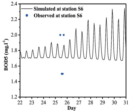
**Figure 19.** Temporal evolution of the simulated and measured of the BOD<sub>5</sub> at point 6 in the case after installation of Kenitra WWTP
