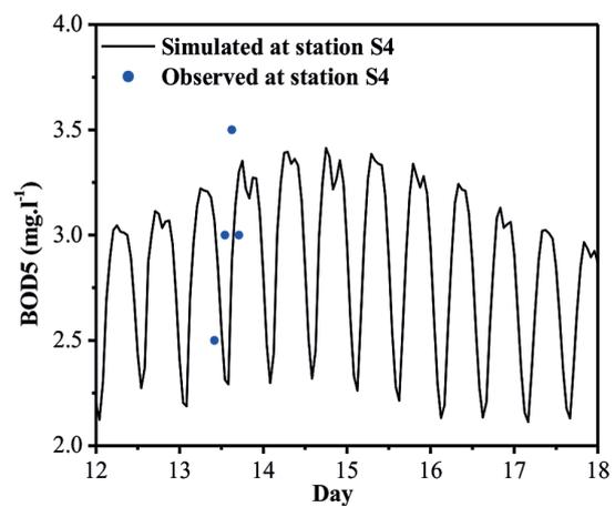
**Figure 17.** Temporal evolution of the simulated and measured of the BOD<sub>5</sub> at point 4 in the case after installation of Kenitra WWTP
