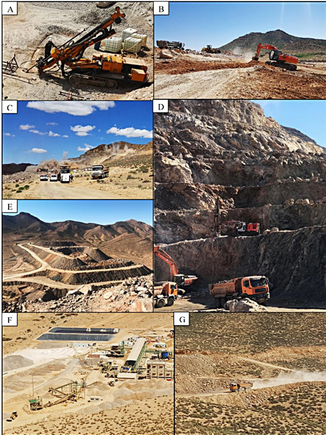
**Figure 2.** Illustration of some mining activities, Jbel Tirremi project, Morocco; A) exploration (drilling and boreholes); B) access tracks; C) blasting; D) open pit method (drilling and loading); E) dumping; F) panoramic view of GFL-GM Fluorspar plant; G) transportation
