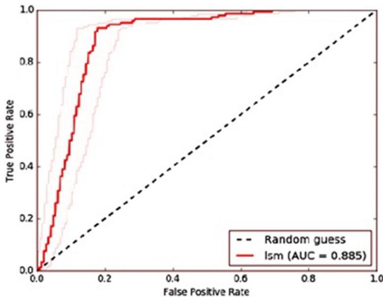
Figure 6. Prediction rate curve for the LSM produced by FAHP model
