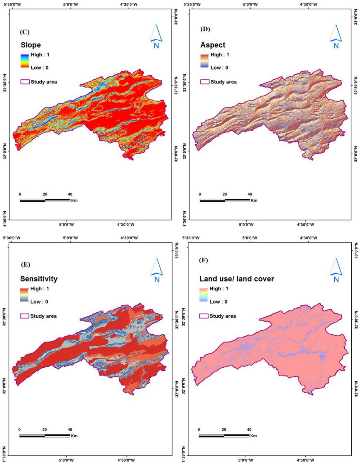
**Figure 3.** Fuzzy map of studied area for each landslide susceptibility parameter: (c) slope, (d) aspect, (e) lithology (sensitivity), (f) LULC
