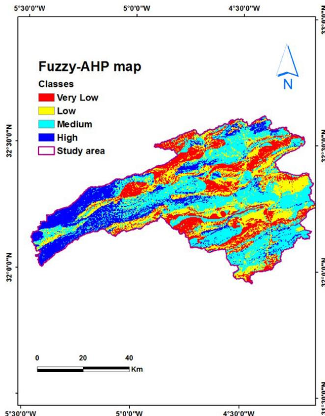
Figure 7. Classified landslide susceptibility map based on FAHP model
