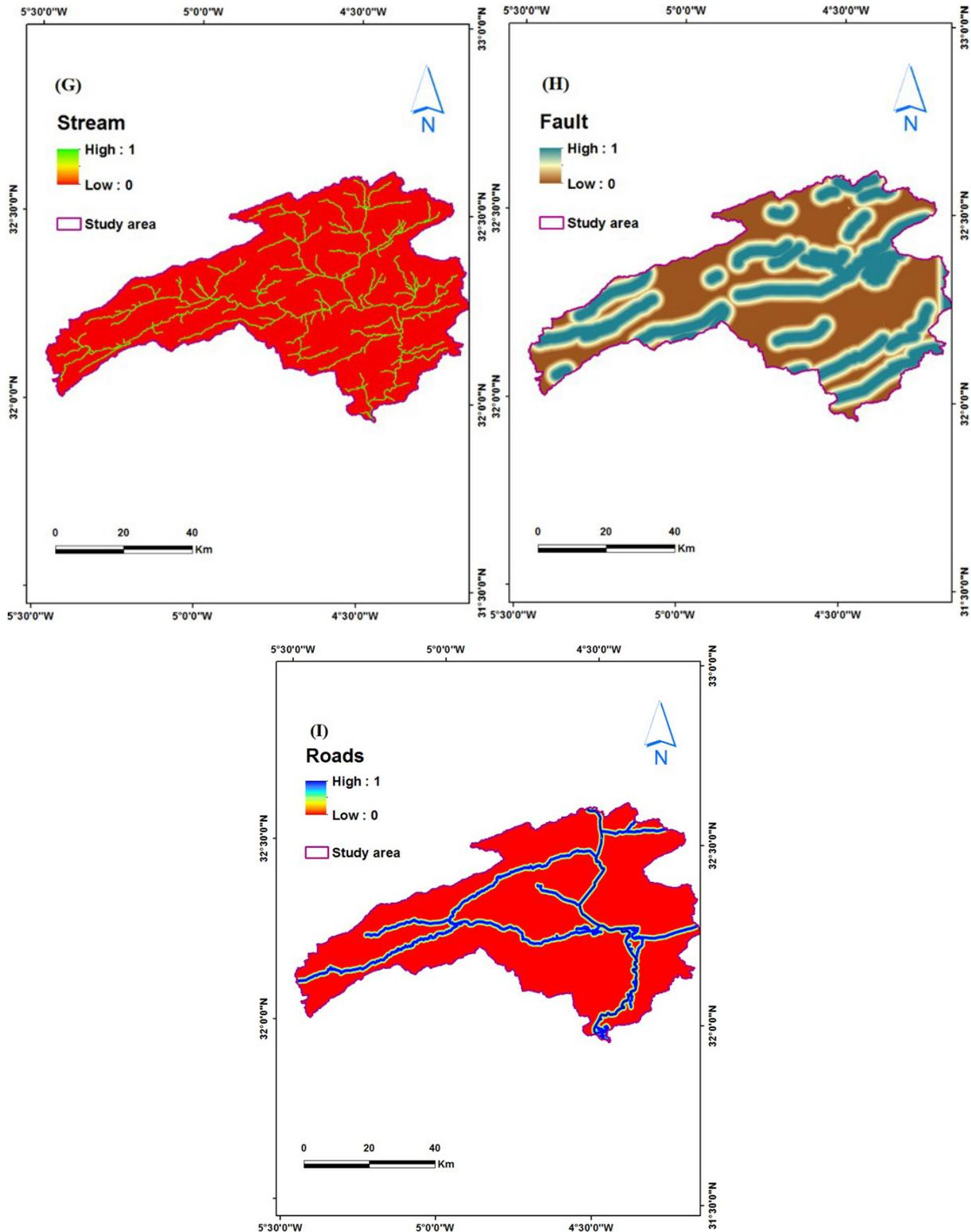
**Figure 3.** Fuzzy map of studied area for each landslide susceptibility parameter: (g) streams, (h), fault, (i) road fuzzy map
