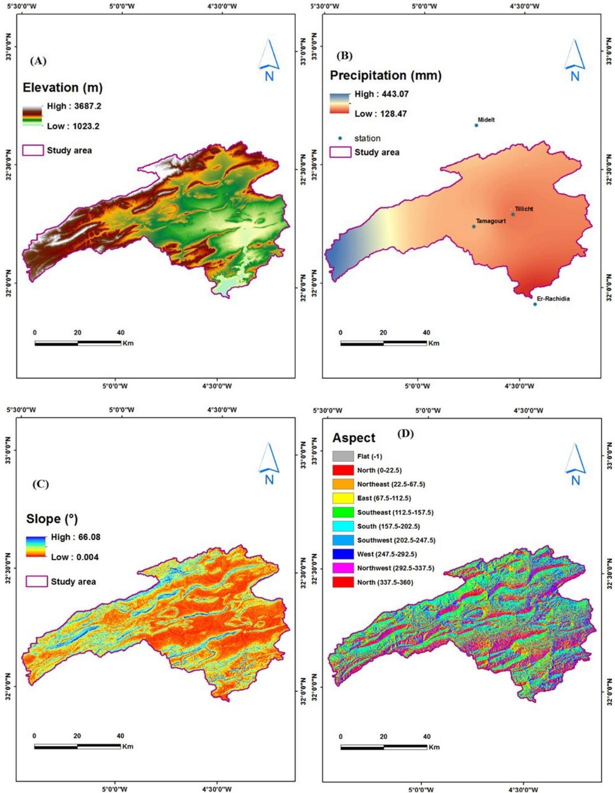
Figure 2. Raster maps used for LSM in this study: (a) DEM, (b) rainfall, (c) slope, (d) aspect
