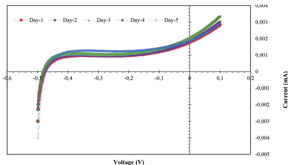
**Figure 9.** Comparison of bioelectricity generation from municipal wastewater collected from STP Salori
