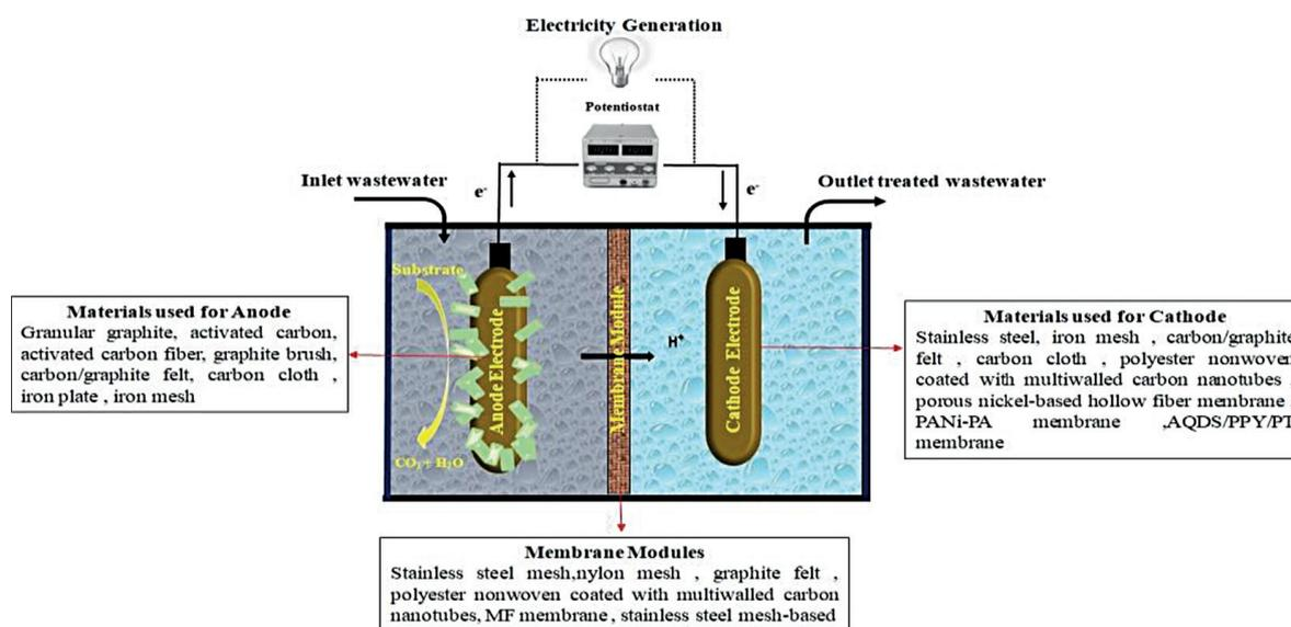
Figure 1. Schematic diagram of EMBR system
