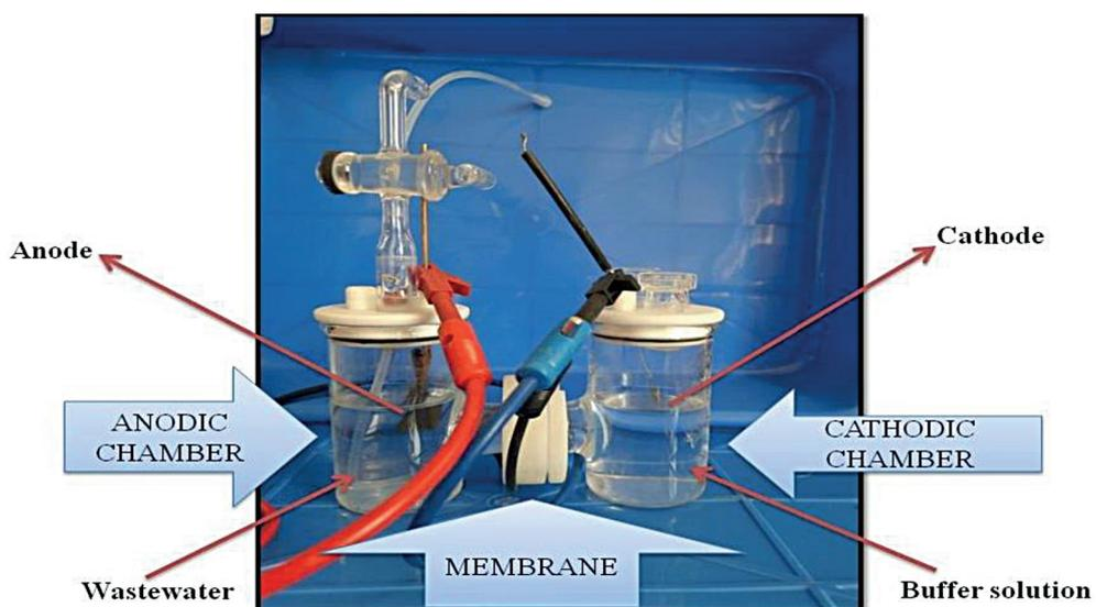
Figure 2. Experimental set-up of EMBR system
