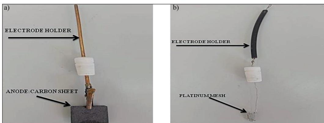
Figure 3. The component of EMBR system: (a) anode (carbon sheet) and (b) cathode (platinum mesh)
