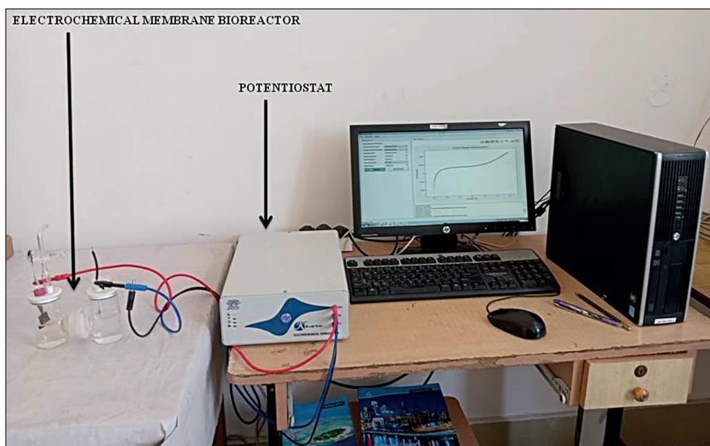
Figure 4. Experimental set up with EMBR and electrochemical potentiostat
