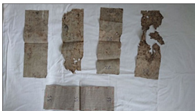
Fig. 1. Specimens of linen cloth after 30 days of exposure in the soil
