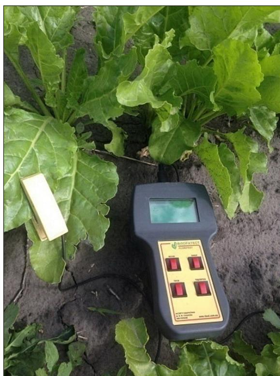
**Fig. 1.** Measurement of chlorophyll fluorescence induction with Floratest
