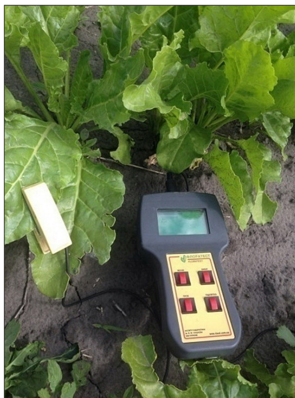
Fig. 1. Measurement of chlorophyll fluorescence induction with Floratest
