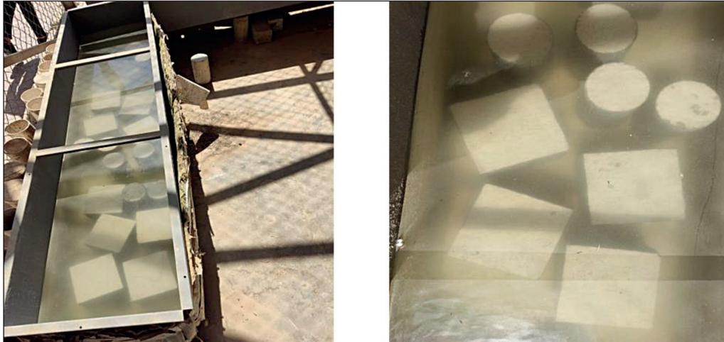
**Figure 6.** Curing process
