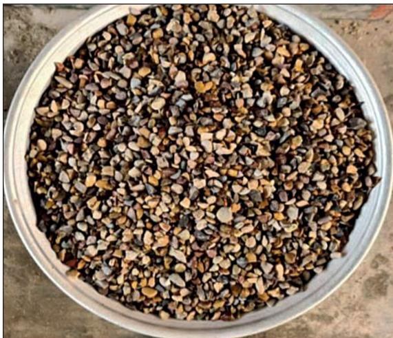
Figure 2. Natural coarse aggregate
