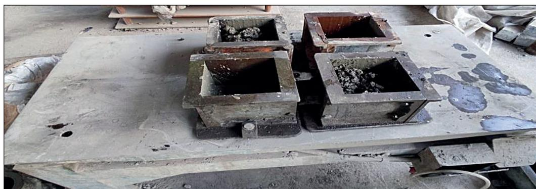
**Figure 4.** Vibrating table
