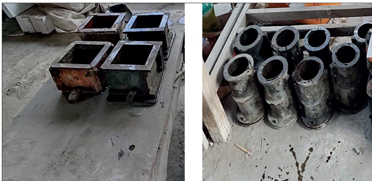
**Figure 3.** Types of specimens
