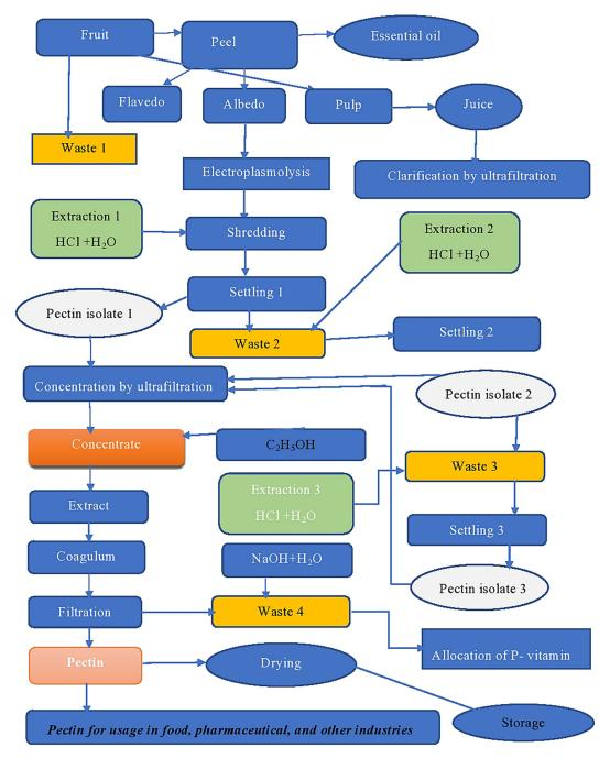
Fig. 7. The technological scheme for obtaining pectin
