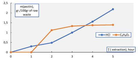
**Fig. 10.** Dependence of isothermal extraction of pectin from fruits of Meer lemon on the time of extraction and the type of extractant (collection date – June 2022, water ratio 1:20, T= 70°C)
