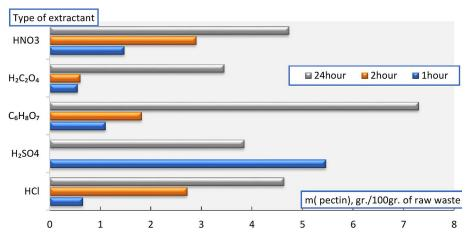
**Fig. 8.** The dependence of the extraction of pectin from the fruit of the Georgian lemon on timeextraction and type of extractant (T(extraction = 20°C), harvest date – May 2022, water ratio 1:20
