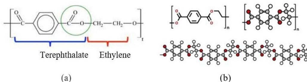
**Figure 1.** Polyethylene terephthalate (PET) Sources (a) Andrady, 2017; (b) Crawford and Quinn, 2017
