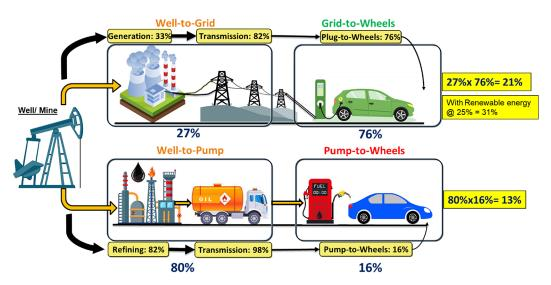
Figure 1. Well to wheel efficiency of ICE vs EVs
