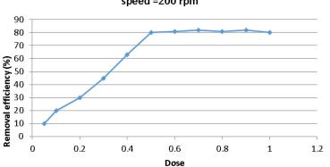
Co=50 mg/L, pH=6, contact Time=130 min, Agitation speed =200 rpm
