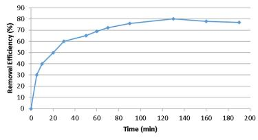
Figure 2. Removal percent of Cu(II) adsorption with contact time
