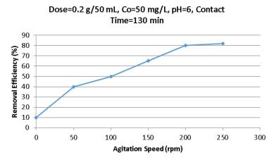
Figure 4. Removal percent of Cu(II) adsorption with agitation speed
