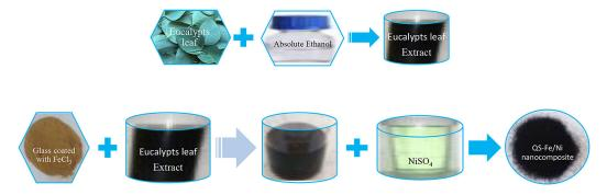
Figure 1. Preparation of Fe/Ni nanocomposite coated sand
