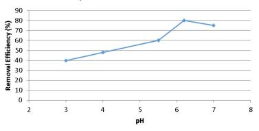
Dose=0.2 g/50 mL, Co=50 mg/L, agitation speed=200 rpm, Contact Time=130 min
