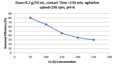
Figure 5. Removal efficiency of Cu(II) adsorption with copper concentration
