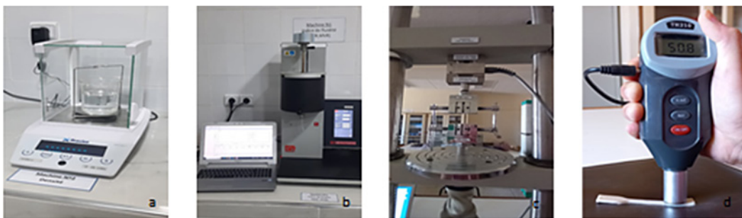
Figure 3. (a) density test, (b) melt flow rate test, (c) tensile strength test, (d) hardness test
