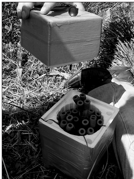
Fig. 3. Temperature in incubation chamber is stable, it is filled with water and allow for fast adjust of temperature. Temperature is set and adjust to constant level for all incubation time using ice cubes or warm water
