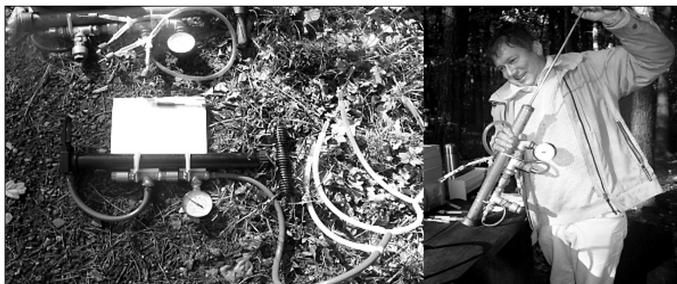
Fig. 2. After sampling leaf rings were placed in test tubes and exposed to low pressure treatment (0.33 atm.). The manual low pressure system is constructed with two valves, vacuumeter and pump with converted piston
