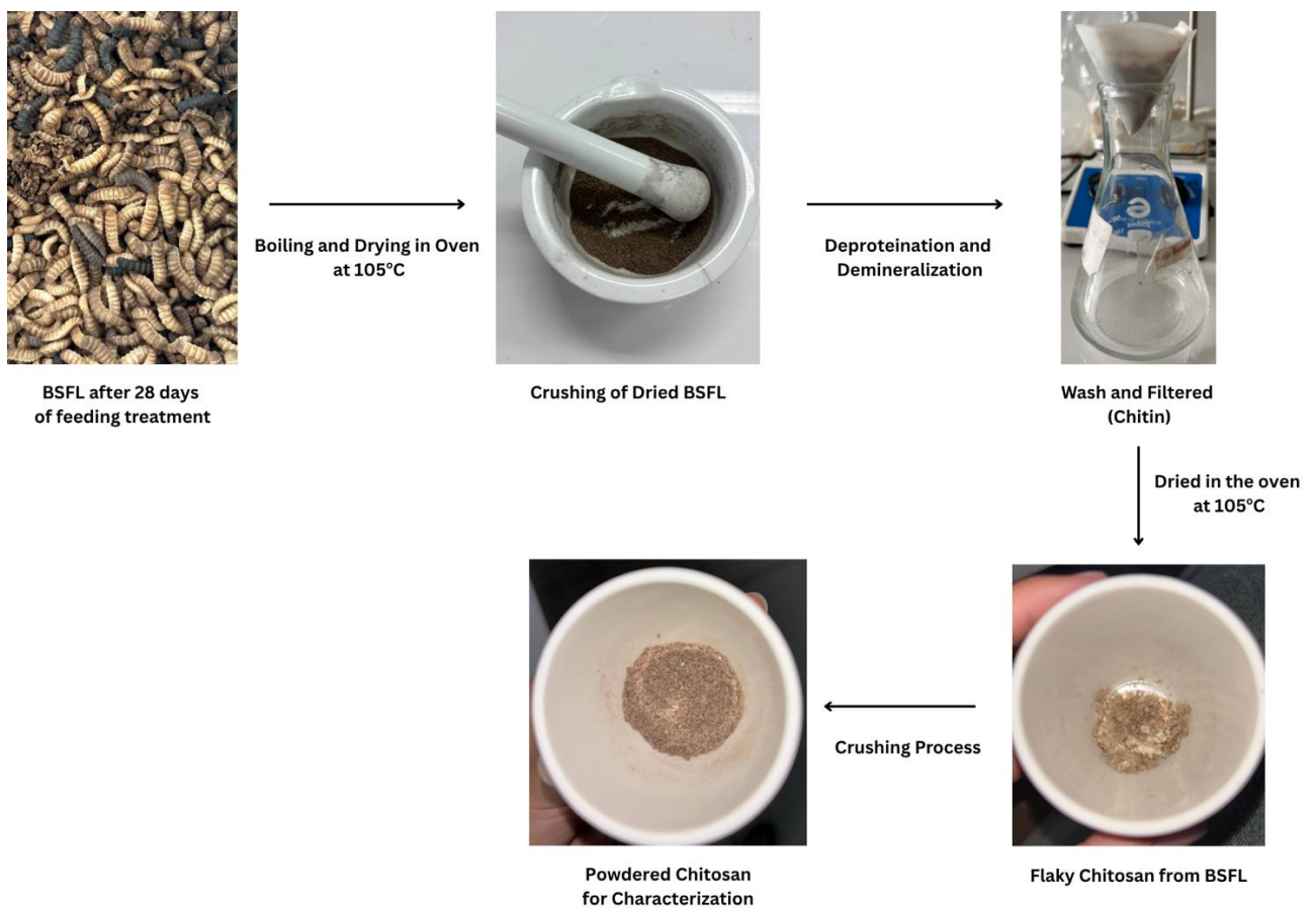
Figure 4S. Step by step larval preparation for chitin extraction and characterization
