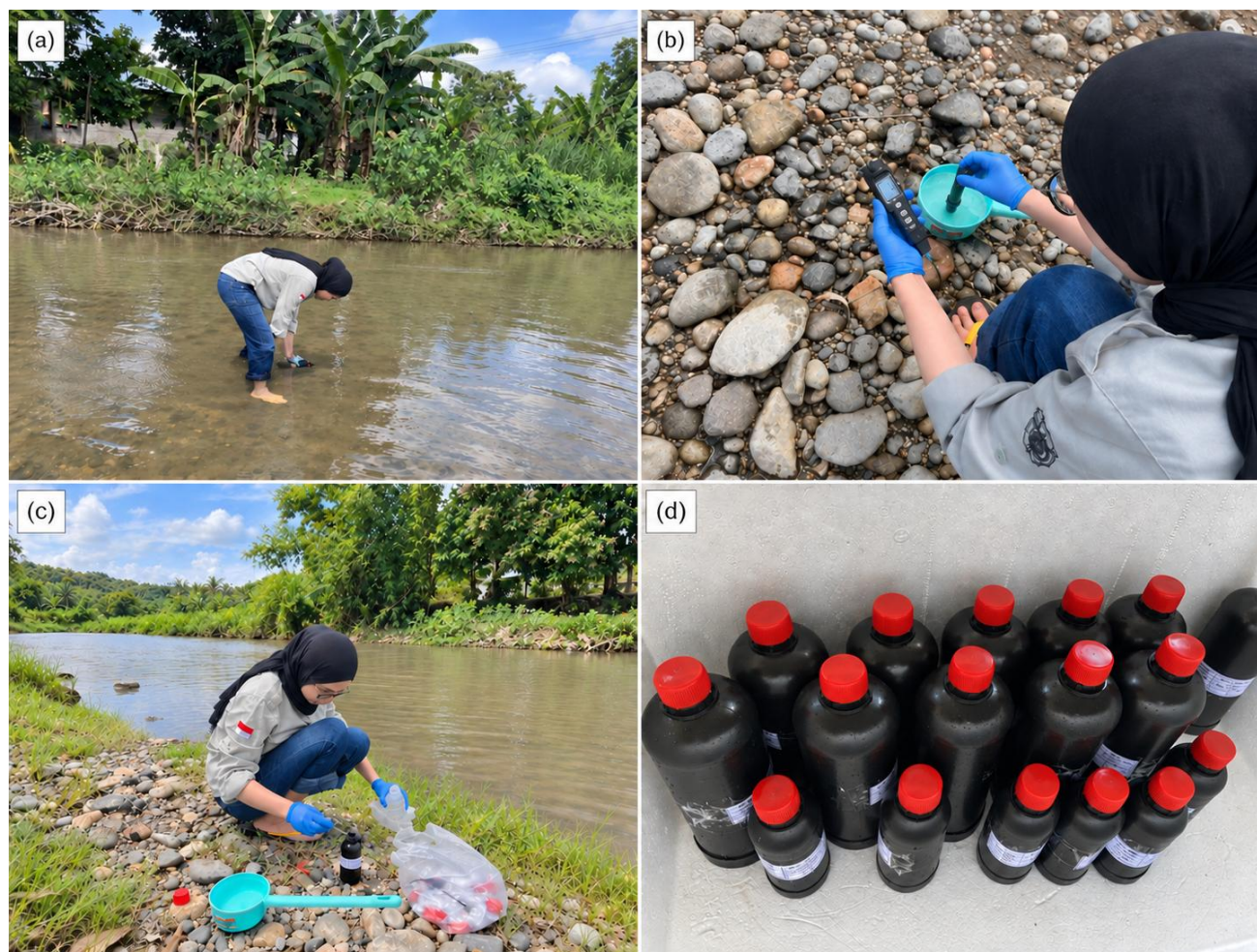
Figure S2. Field water sampling and sample handling procedures in the Biyonga River: (a) water sampling, (b) in situ water quality measurement, (c) sample preparation and handling, and (d) collected water samples.
