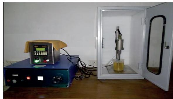
Figure 3. Ultrasonic sonicator
