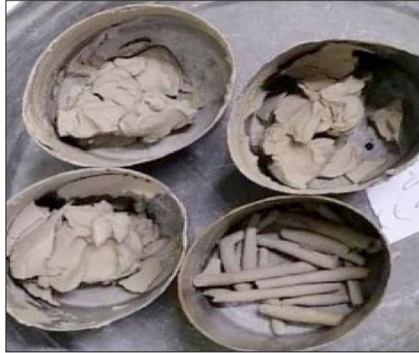
Figure 4. Atterberg limits test
