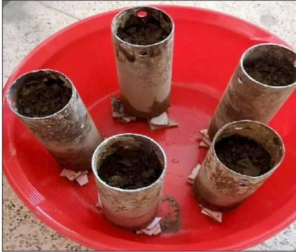
Figure 2. Undisturbed soil samples
