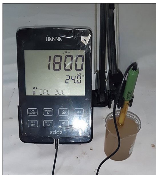
Figure 3. Themultiparameter sensor used in effluents analyses
