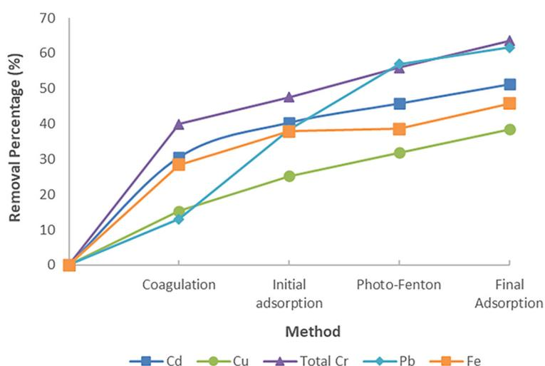
Figure 5. Heavy metals reduction after treatment method
