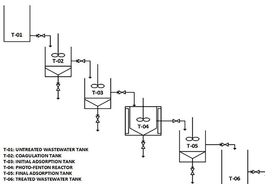
Figure 1. The prototype of laboratory wastewater treatment
