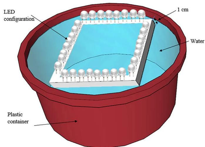
**Figure 7.** Light trap with LEDs at 1 cm from the water
