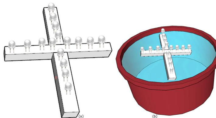
**Figure 5.** 16-LED cross configuration: (a) positioning of the LEDs and b) location on the water
