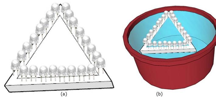
**Figure 4.** 24-LED triangle configuration: (a) positioning of the LEDs and (b) location above the water
