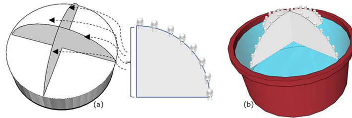
**Figure 2.** Semi-spherical configuration of 32 LEDs: (a) positioning of the LEDs and (b) location above the water
