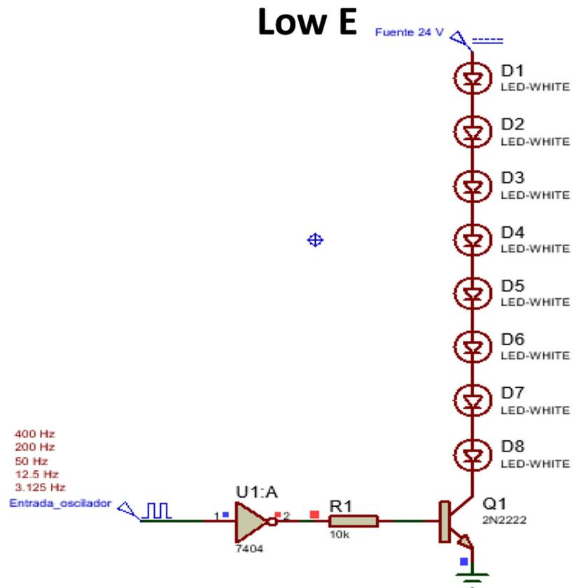
**Figure 6.** Switching and luminescence control circuit of the different LED configurations
