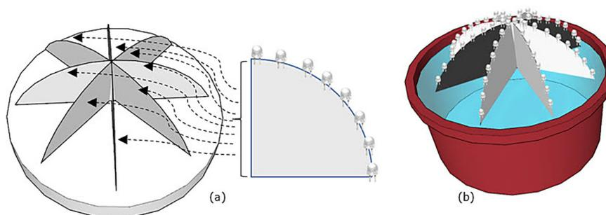
**Figure 1.** 64-LED hemispherical configuration: (a) LED positioning and (b) location above the water
