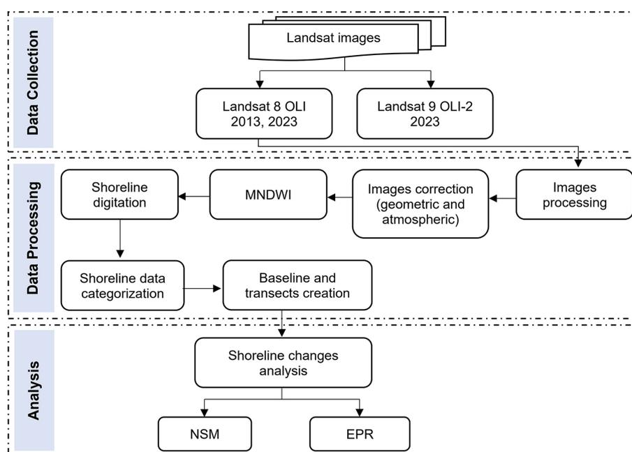
**Figure 2.** Flowchart of the process of identifying and determining shoreline changes from multitemporal satellite imagery: processing and analysis of satellite imagery
