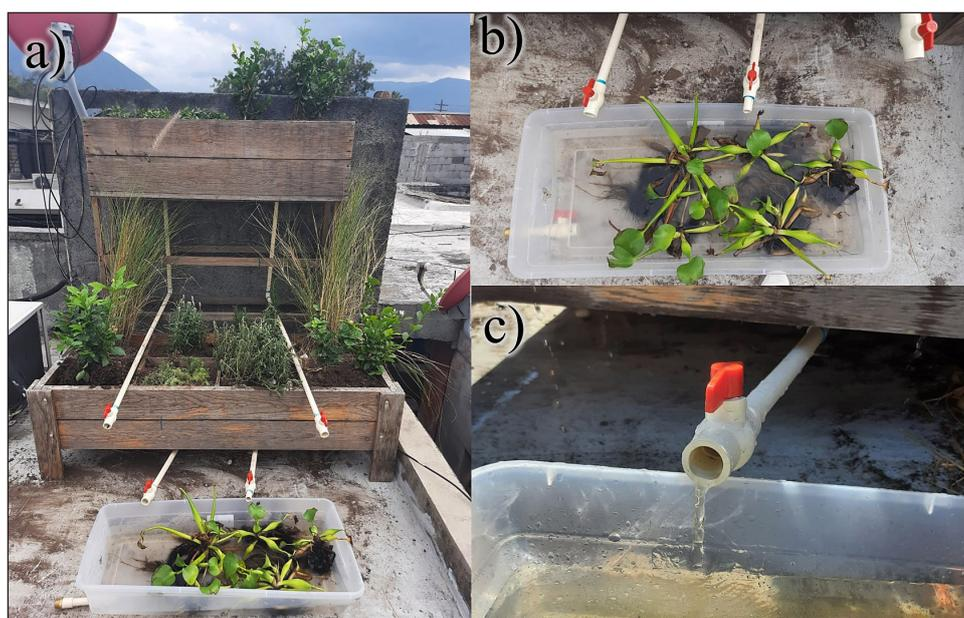
**Fig. 1:** a) Complete green infrastructure prototype (roof, wall, and wetland), b) wetland prototype, c) water excreted towards the wetland prototype
