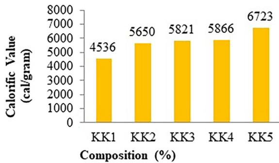
Figure 9. Charcoal briquettes calorific value
