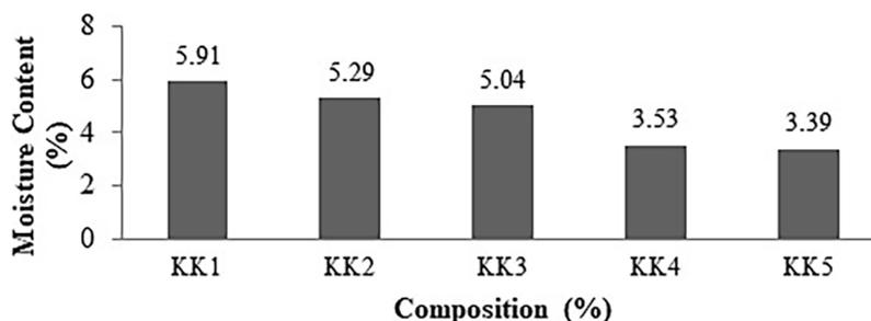
Figure 2. Moisture content of charcoal briquettes
