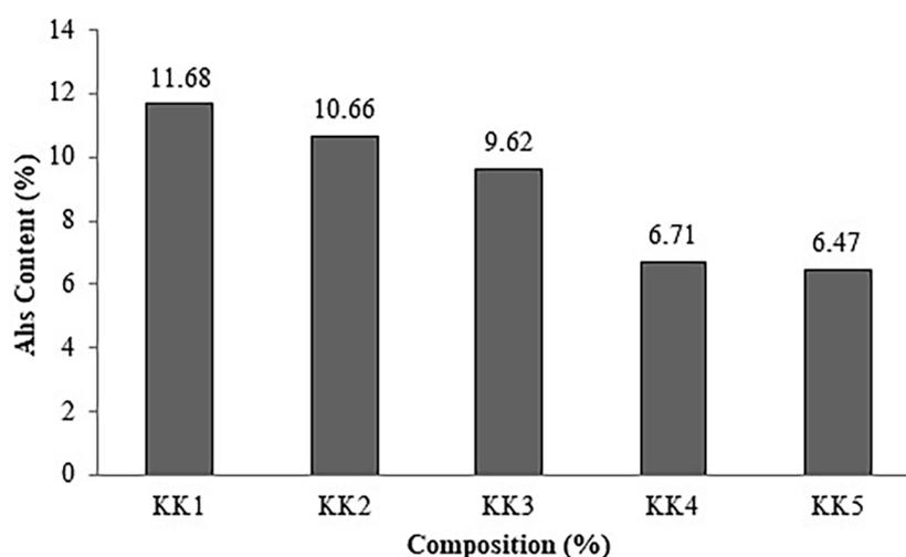
Figure 4. Ash content of charcoal briquettes
