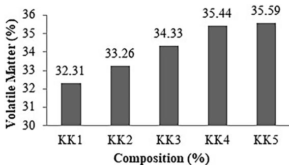
Figure 6. Volatile matter from charcoal briquettes
