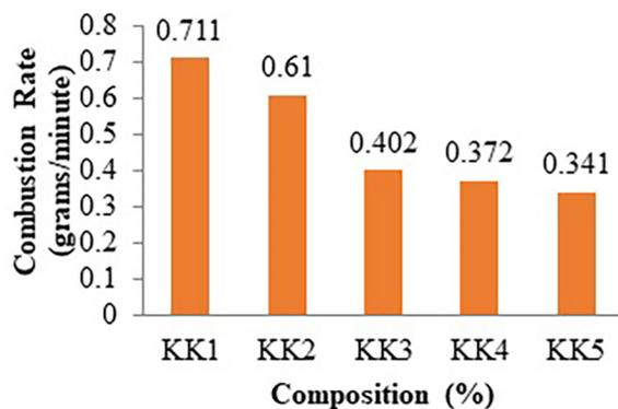
Figure 10. Burning rate of charcoal briquettes
