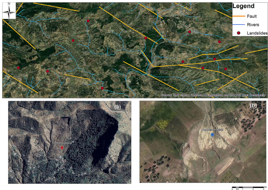
Figure 8. A map displaying landslides near faults and rivers: (a) near a fault and (b) near a stream
