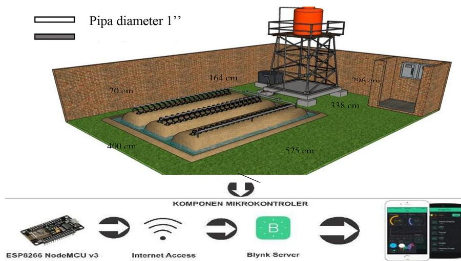
**Fig. 1.** IoT-based drip irrigation system design
