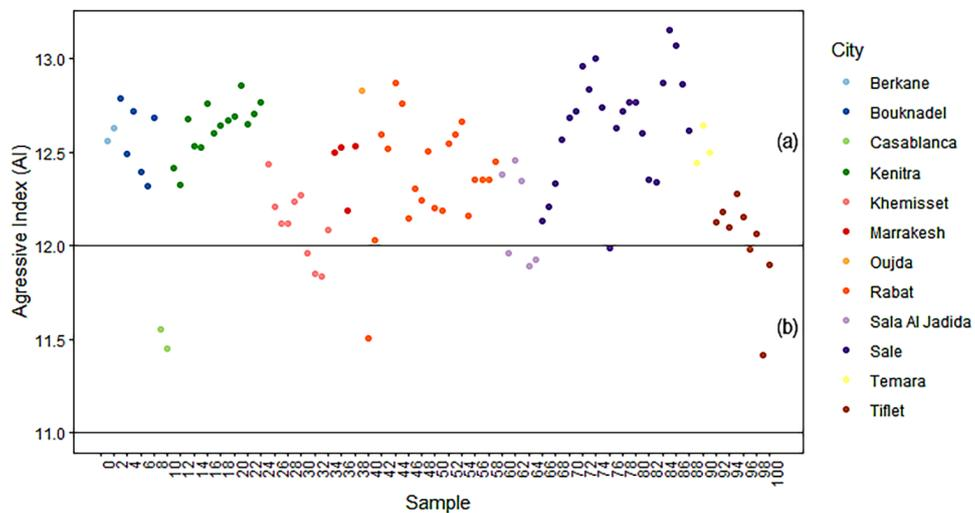
**Figure 5.** Values of the calculated aggressive index (AI) for each sample and city. (a) Non-aggressive water, (b) Moderately aggressive water
