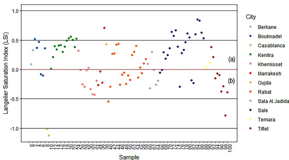
**Figure 2.** Values of the calculated Langelier saturation index (LSI) for each sample and city. (a) Water is supersaturated and likely to scale when the LSI is positive. (b) Water is undersaturated and tends to be corrosive when the LSI is negative
