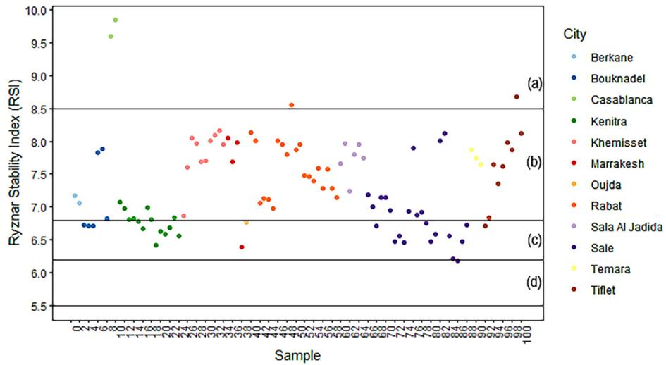
**Figure 3.** Values of the calculated Ryznar stability index (RSI) for each sample and city. (a) Very corrosive water, (b) Corrosive water, (c) Stable water, (d) Scaling water
