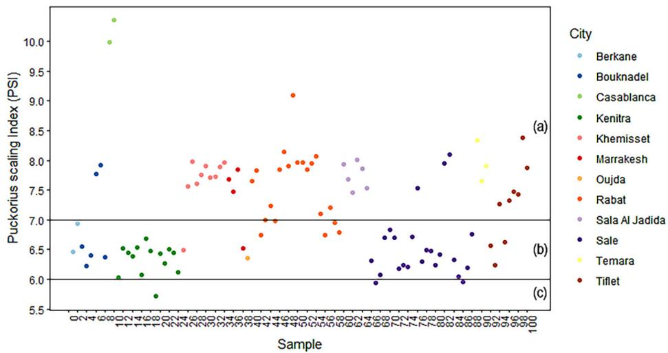
**Figure 4.** Values of the calculated Puckorius scaling index (PSI) for each sample and city. (a) and (b) Water is undersaturated and tends to be corrosive, (c) Water is supersaturated and tends to scale
