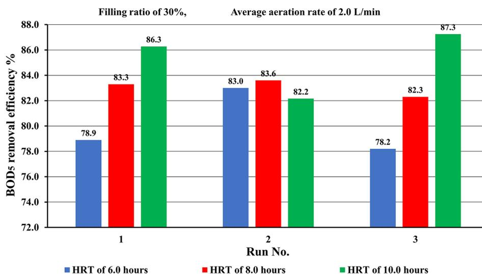
Figure 6. BOD<sub>5</sub> removal efficiency at different HRTs
