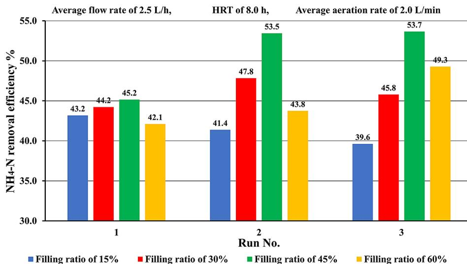
Figure 5. NH<sub>4</sub><sup>+</sup>-N removal efficiency at different filling ratios
