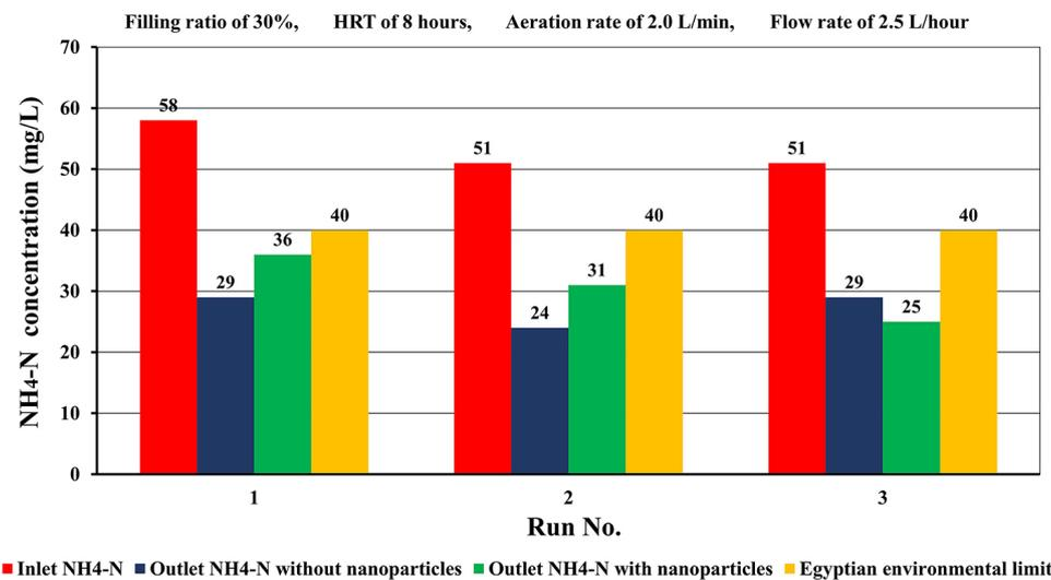
Figure 11. Inlet and outlet NH<sub>4</sub><sup>+</sup>-N concentration of MBBR with and without nanoparticles compared with Egyptian environmental low limits of low 48 for year 1982
