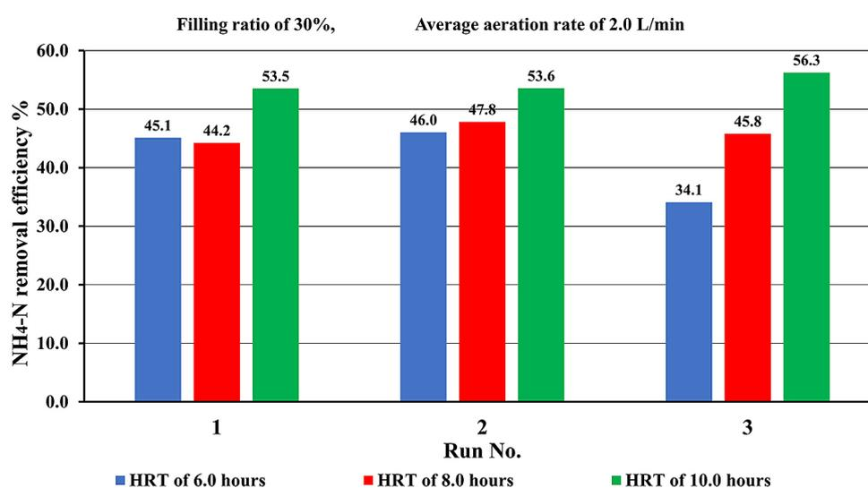
Figure 8.  $\text{NH}_4^+\text{-N}$  removal efficiency at different HRTs
