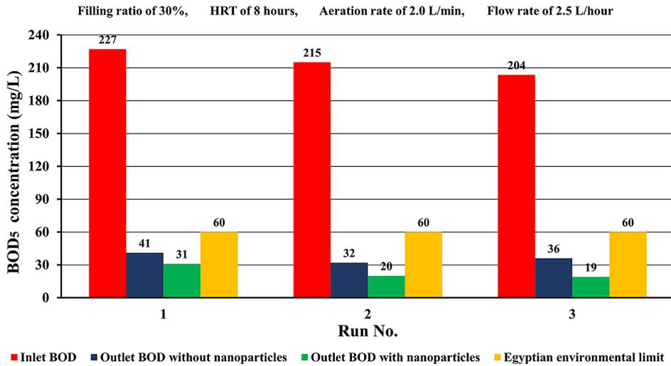
Figure 9. Inlet and outlet BOD<sub>5</sub> concentration of MBBR with and without nanoparticles compared with Egyptian environmental low limits of low 48 for year 1982
