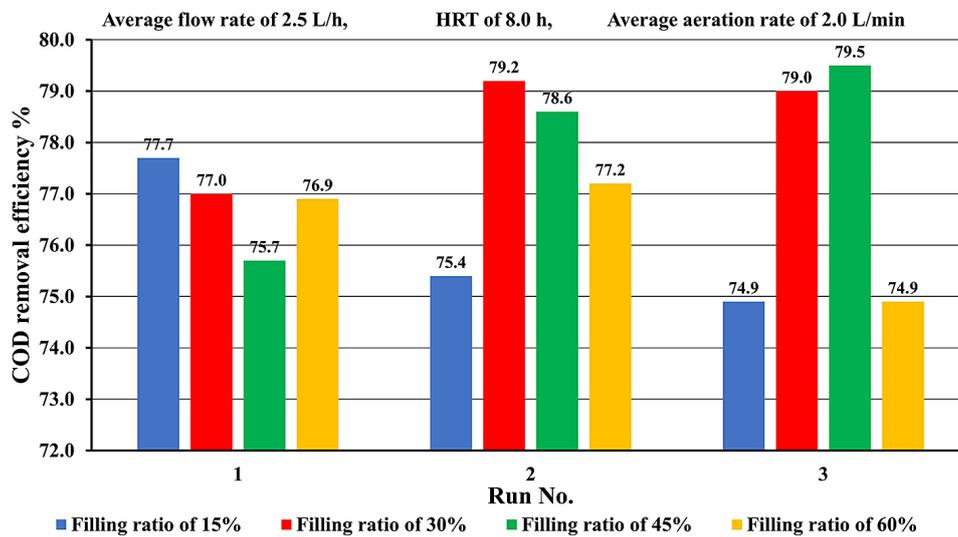
Figure 4. COD removal efficiency at different filling ratios
