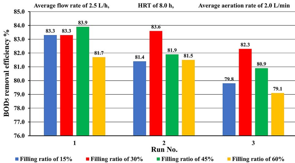
Figure 3. BOD<sub>5</sub> removal efficiency at different filling ratios
