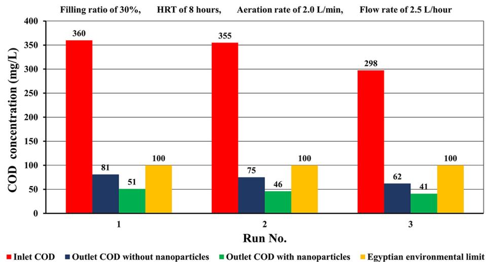
Figure 10. Inlet and outlet COD concentration of MBBR with and without nanoparticles compared with Egyptian environmental low limits of low 48 for year 1982
