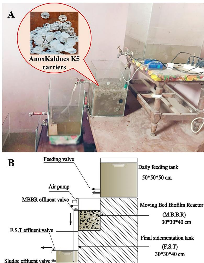
**Figure 2.** Experimental setup of MBBR system followed by settling tank in (a) a photo image, (b) a schematic diagram
