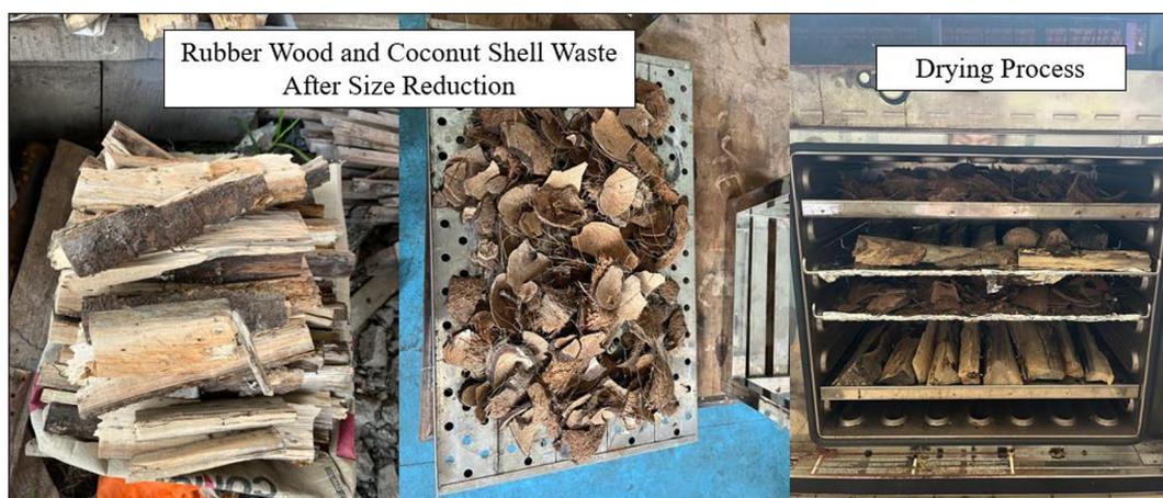
Figure 3. The pre-treatment of raw material
