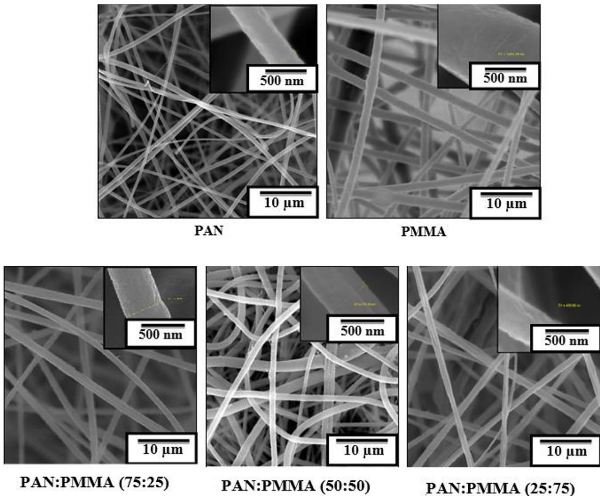
Figure 4. SEM of double-layer nonwoven nanofiber membranes (PAN: PMMA) that were prepared after MD experiments with thickness (10 µm)
