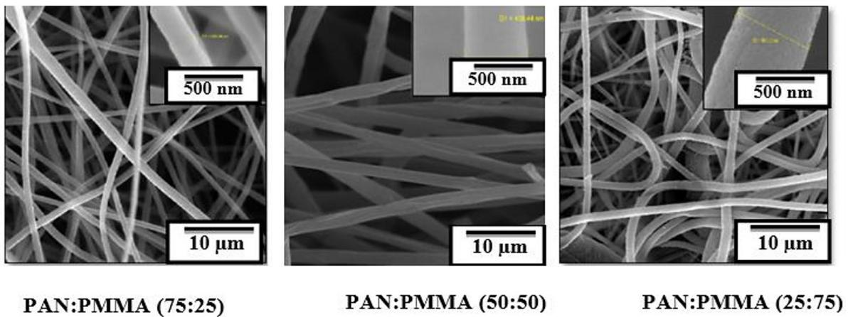
**Figure 3.** SEM of double-layer nonwoven nanofiber membranes (PAN: PMMA) that were prepared before MD experiments with the thickness (10 µm)
