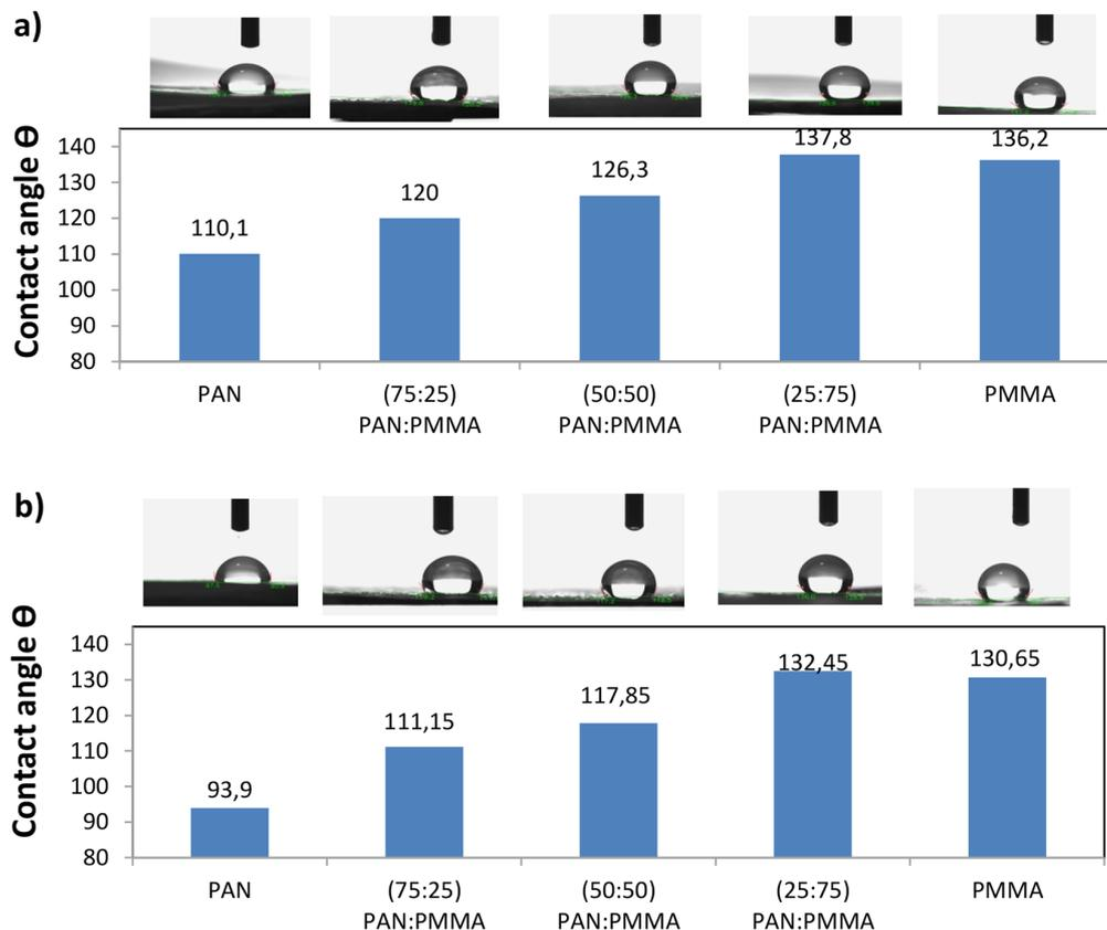
**Figure 5.** Contact angle of the obtained double-layers (PAN: PMMA) membranes of nanofibers nonwoven before and after MD experiments (a) before MD (b) after MD
