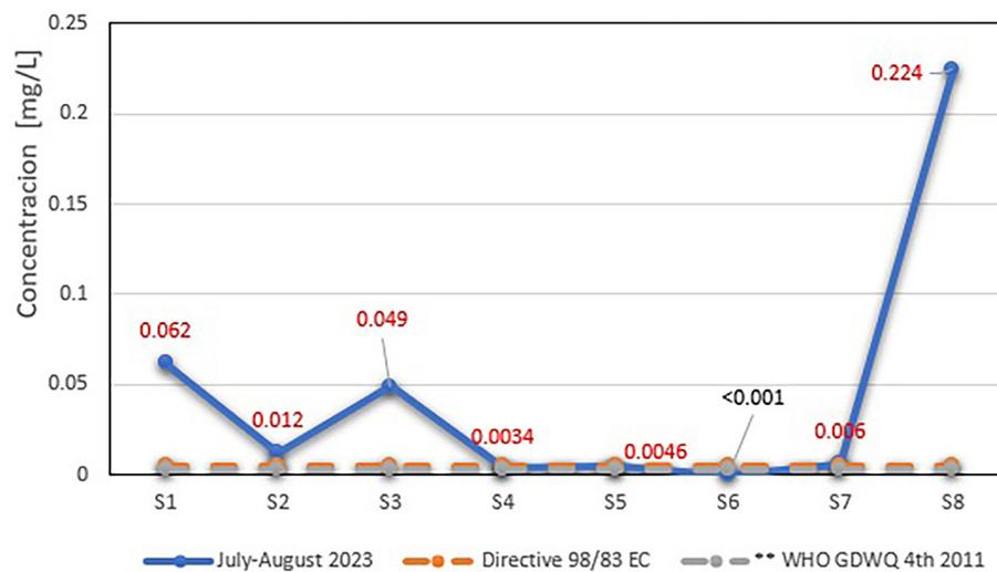
Figure 11. Cadmium concentration according to sampling points
