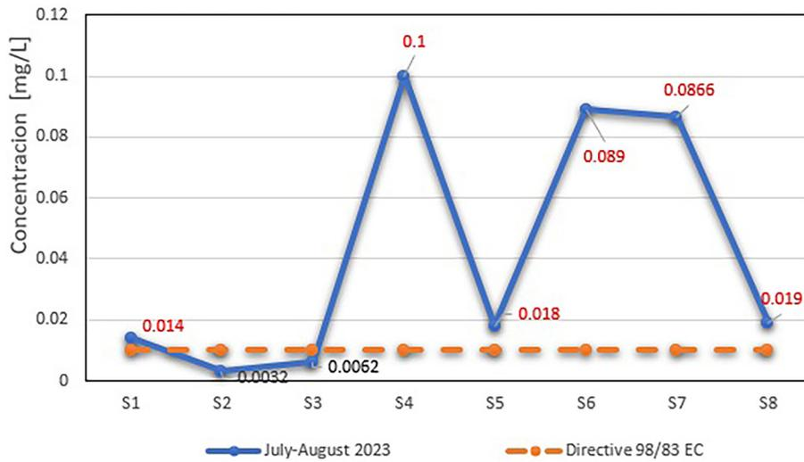
Figure 9. Lead concentration according to sampling points
