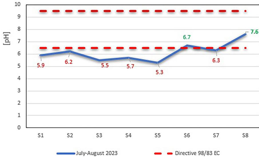
Figure 3. H<sup>+</sup> ion concentration according to sampling points
