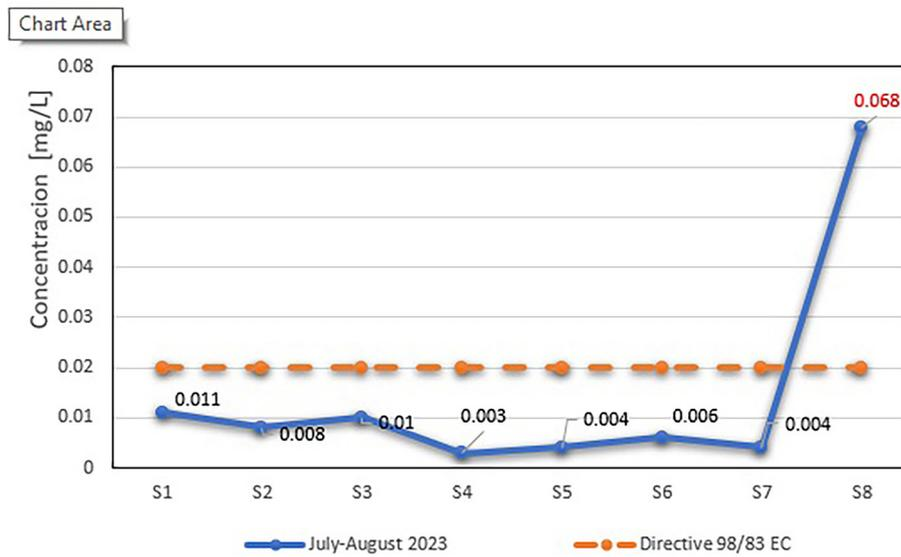
Figure 10. Nickel concentration according to sampling points
