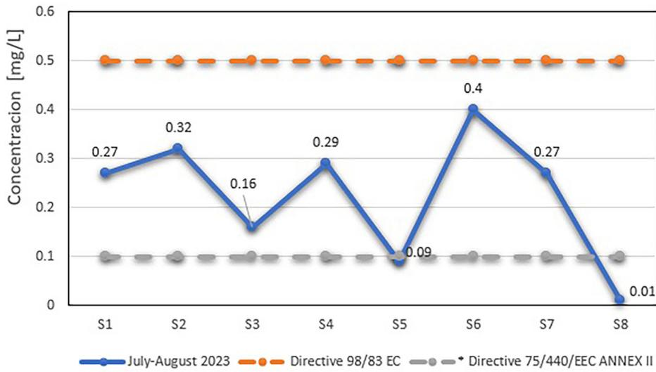
Figure 5. Amonium  $\text{NH}_4^+$  concentration according to sampling points
