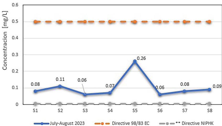
Figure 7. Nitrites  $\text{NO}_2^-$  concentration according to sampling points
