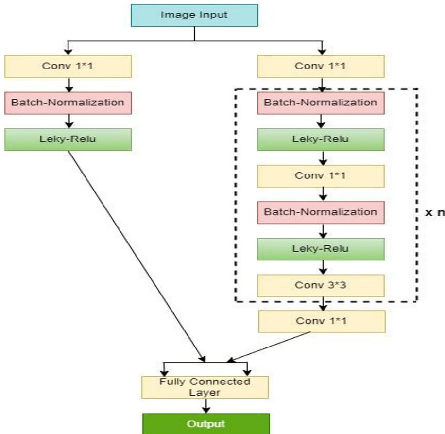
**Figure 7.** Backbone training architecture of CSP-DarkNet-53
