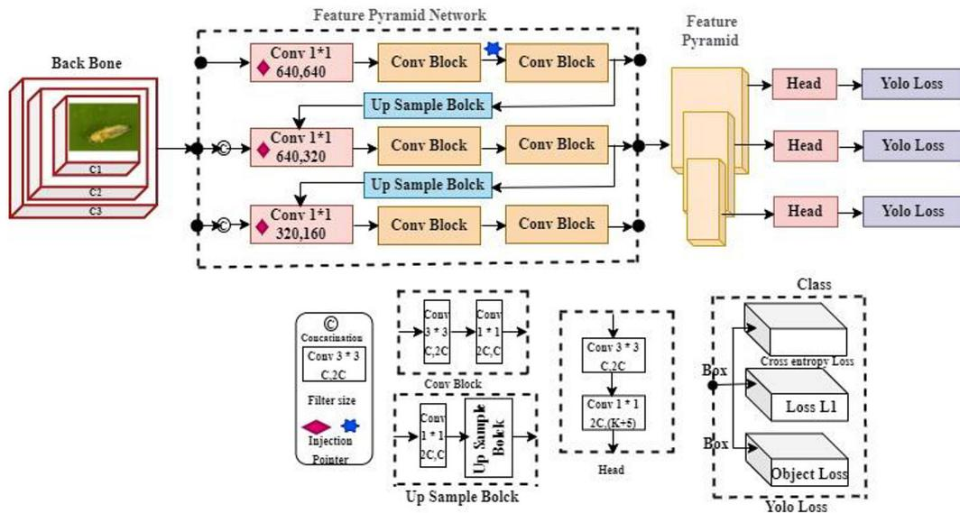
Figure 10. Layered architecture of Yolo v7 architecture for pest class
