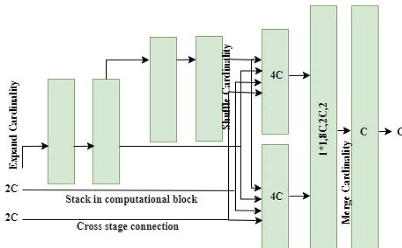
Figure 9. YOLOv7 (E-ELAN) backbone architecture
