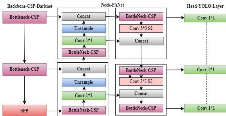
Figure 6. YOLOv5 architecture with CSP-DarkNet(Backbone), PANet(Neck) and yolo layer (head)
