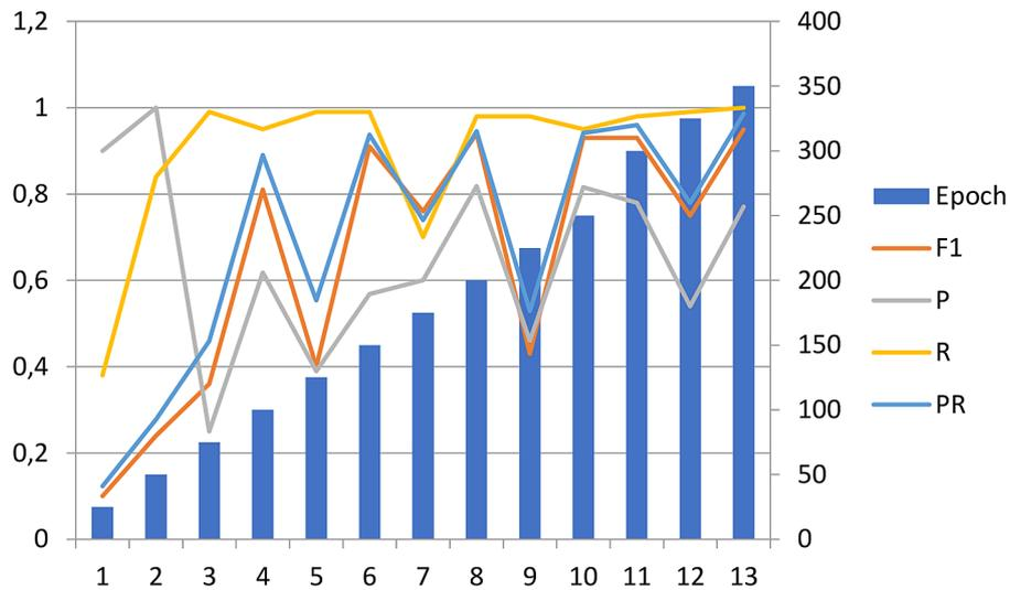
Figure 21. Performance analysis YOLOv5s of F1-Score, precision, recall, precision-recall with respect to epochs
