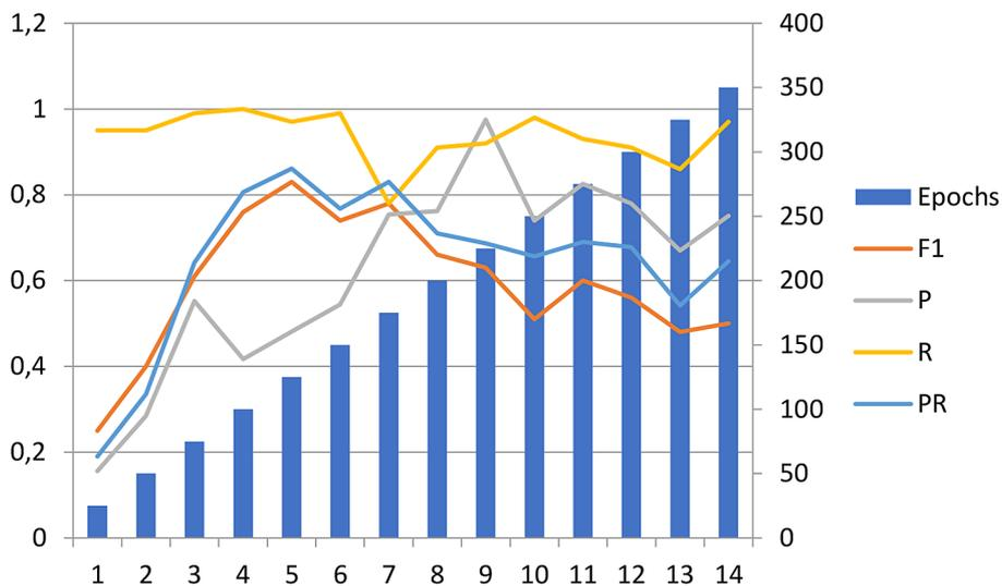
Figure 22. Performance analysis YOLOv7 of F1-Score, precision, recall, precision-recall with respect to epochs
