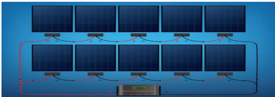
Fig. 5. Example of two chains of panels in series, which are connected parallelly to a string grid inverter. Each chain is constituted of 5 panels (taken from: www.energy2Store.hr/en/ )
