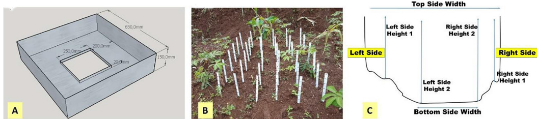
Figure 2. Illustration of soil erosion measurements: a) splash cup (splash erosion); b) pin erosion(sheet erosion); and c) volumetric methods (rill and gully)
